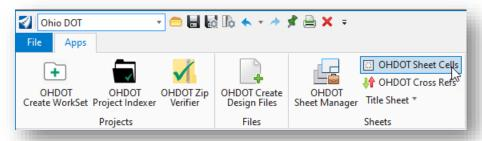
Cells that have interior components, such as the title sheet, are split into two separate cells: one for the border and one for the interior. Placement of the sheet cell border and interior is facilitated by use of the **OHDOT Sheet Cells** application.
