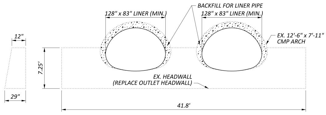
EX. INLET/OUTLET HEADWALL DETAIL (NOT TO SCALE)
