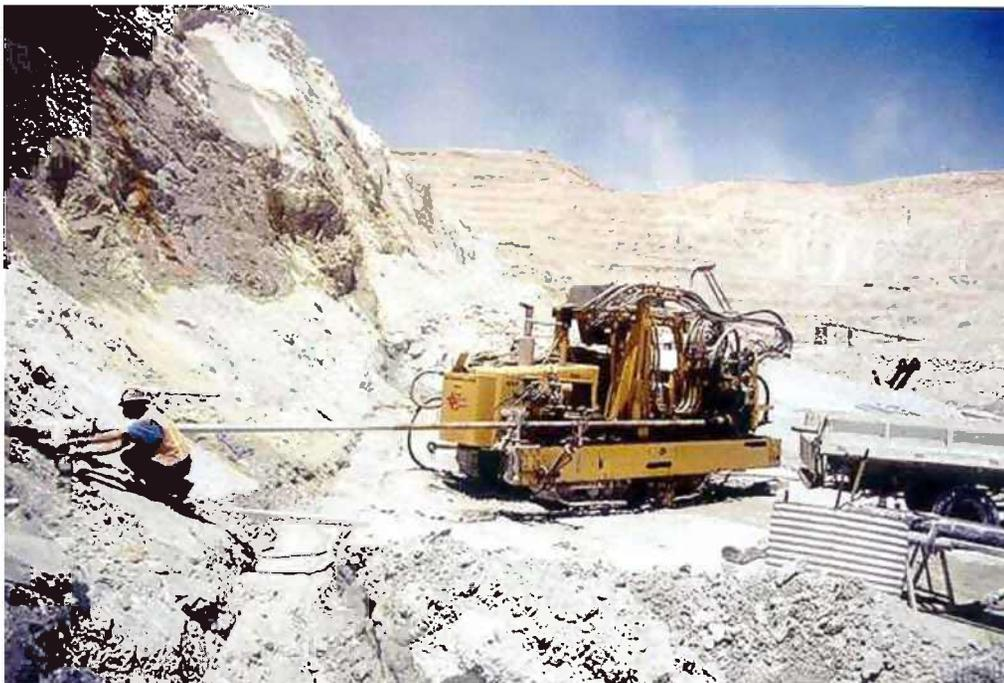
**Figure 8.2: Pictures of horizontal drain installation equipment**
