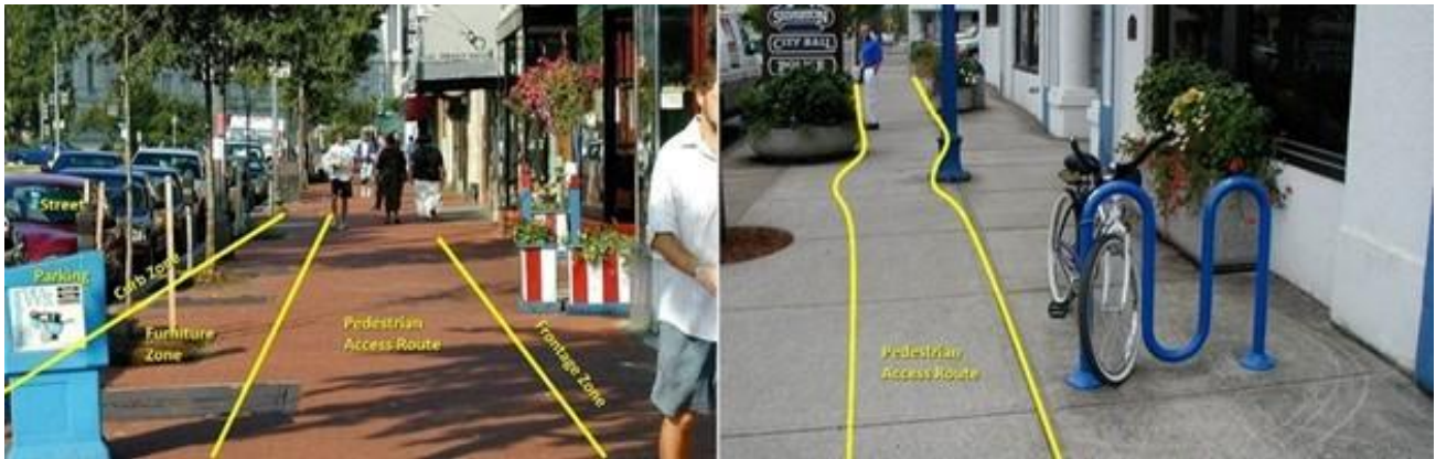
Figure 4-4: Photos showing an accessible and intuitive Pedestrian Through Zone versus a compliant but unintuitive Pedestrian Through Zone
