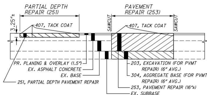
**PAVEMENT REPAIR DETAIL**
