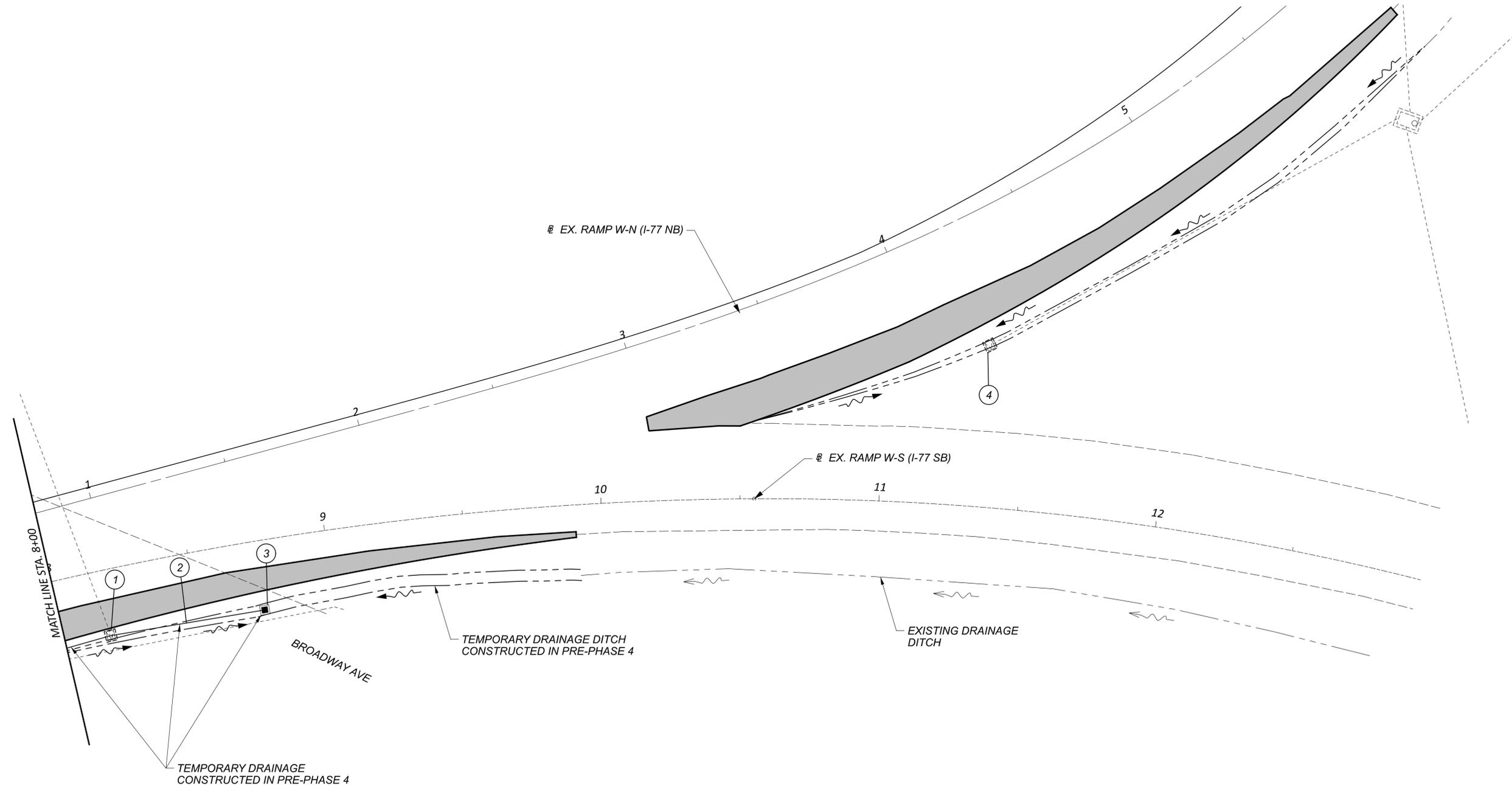
TEMPORARY DRAINAGE CONSTRUCTED IN PRE-PHASE 4
