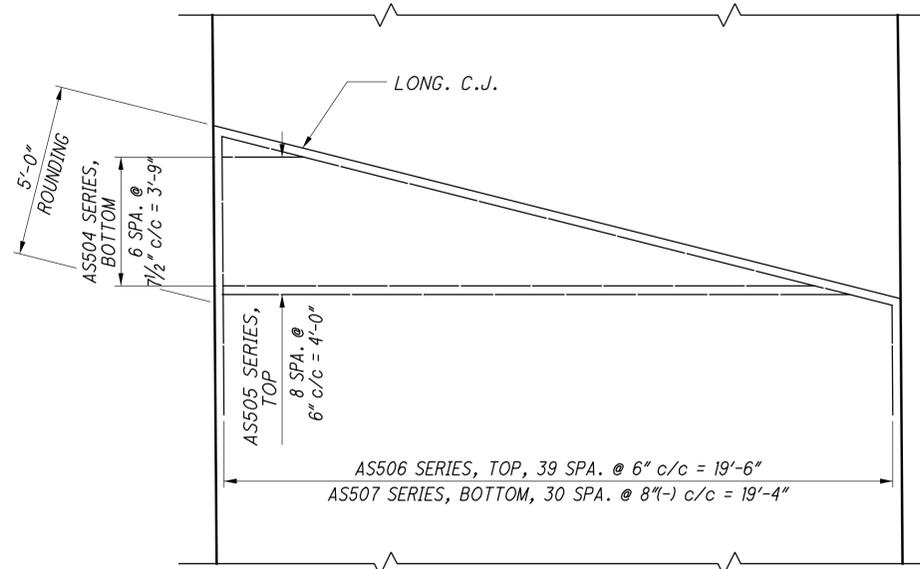
PART PLAN - REAR APPROACH SLAB REINFORCING
