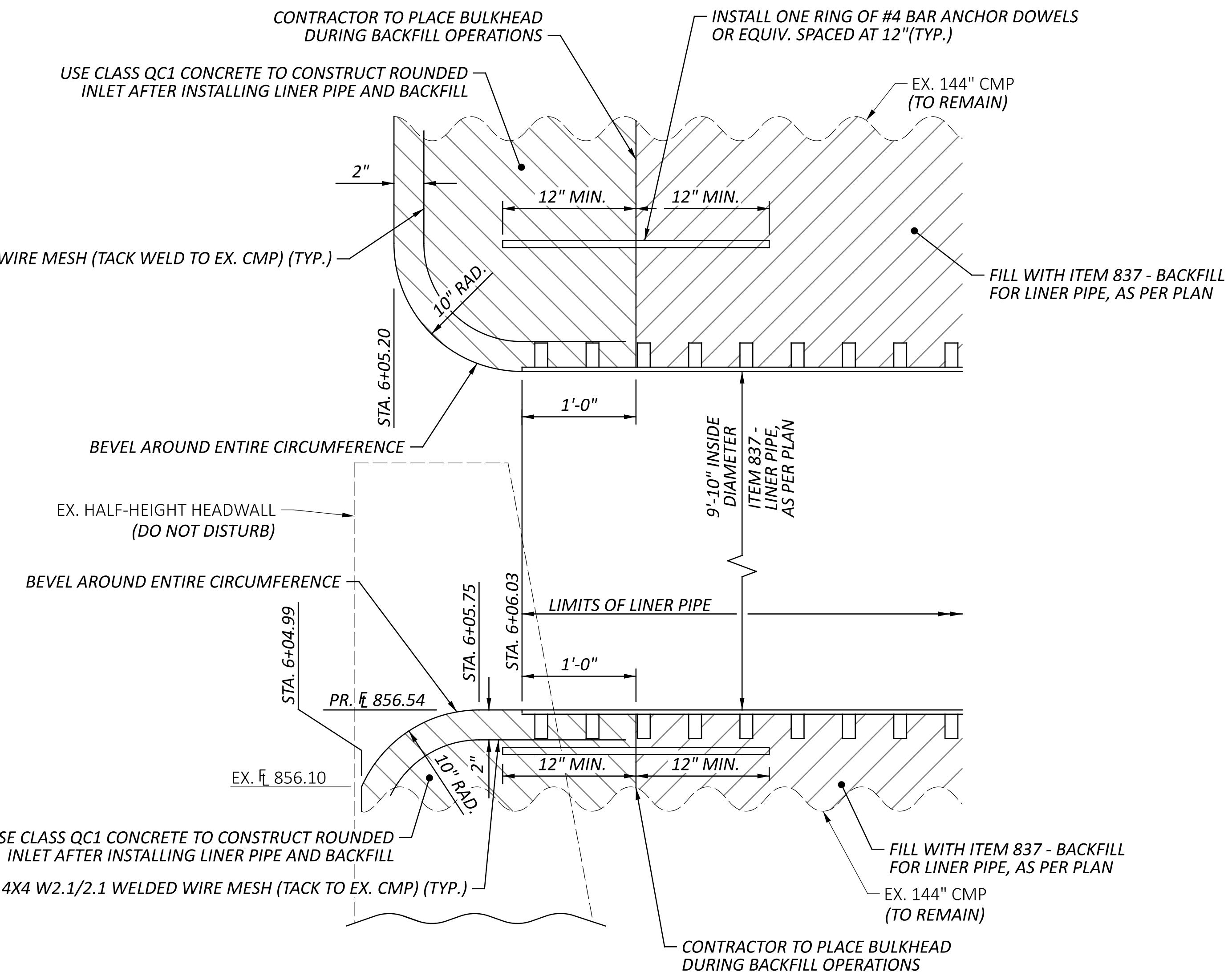
CULVERT INLET DETAIL - PROFILE VIEW
