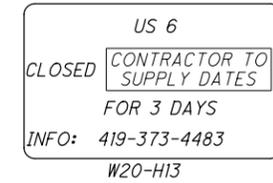
THE CONTRACTOR SHALL PROVIDE, ERECT AND MAINTAIN STANDARD 48 X 30 INCH (1200 X 750 MILLIMETERS) ROAD CLOSED SIGNS, SIGN SUPPORTS, BARRICADES AND LIGHTS AS DETAILED ON SCD MT-101.60, DURING PERIODS IN WHICH THE AFFECTED ROADS ARE CLOSED TO TRAFFIC.
