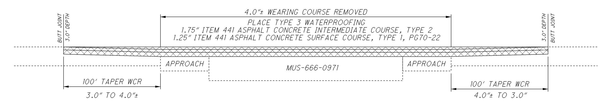
REMOVE 4.0"± ASPHALT CONCRETE, WATERPROOFING AND DRIP STRIP PLACE WATERPROOFING, DRIP STRIP AND 3.0" ASPHALT CONCRETE
