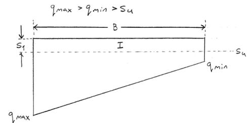
Unit Shear Resistance for Case 4:
