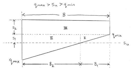
Unit Shear Resistance for Case 2:
