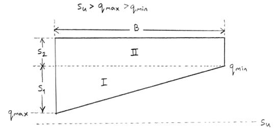
Unit Shear Resistance for Case 3:
