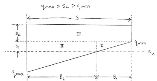
Unit Shear Resistance for Case 2:
