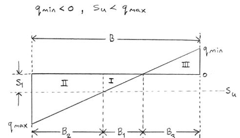
Unit Shear Resistance for Case 5:
