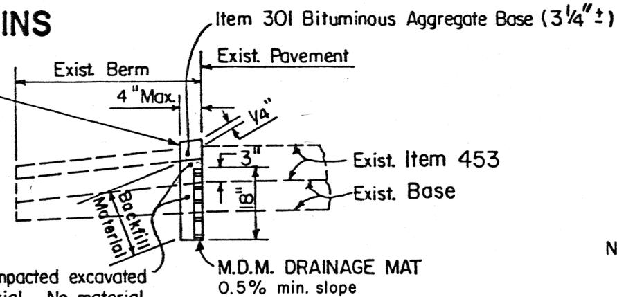
Recompacted excavated material. No material over 2 1/2" in size will be permitted.
