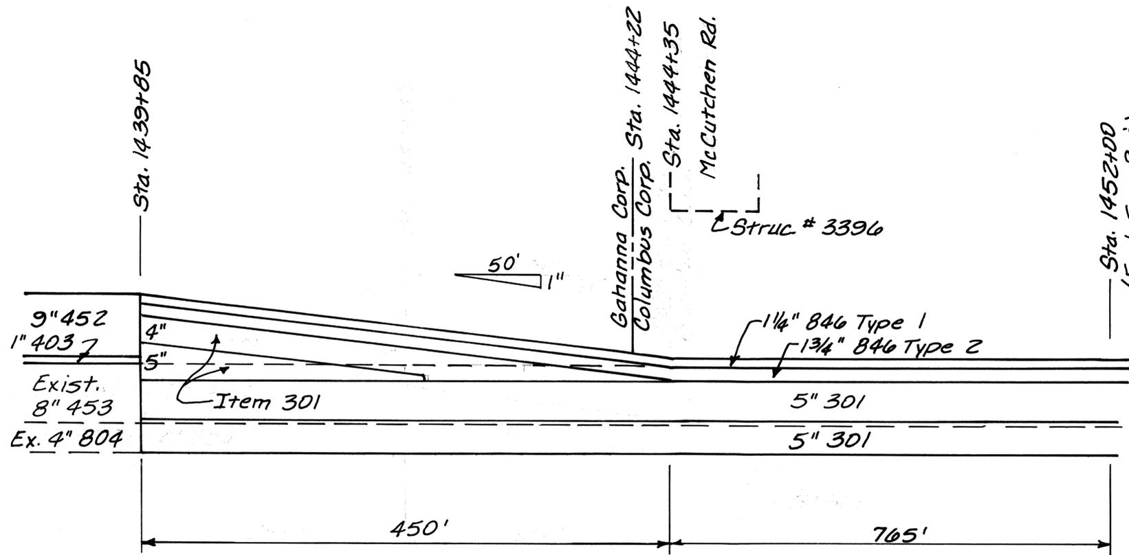
DETAIL AT TRANSITION FROM CONCRETE OVERLAY (Sec. B) TO FULL DEPTH REPLACEMENT
