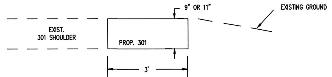
ITEM 451 - 9" Reinforced Concrete Pavement, as per plan
