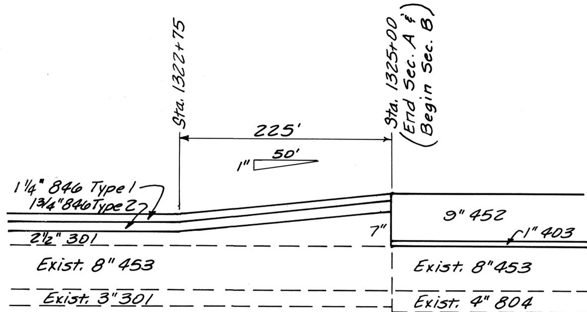
DETAIL AT TRANSITION FROM ASPHALT OVERLAY (Sec. A) TO CONCRETE OVERLAY (Sec. B)
