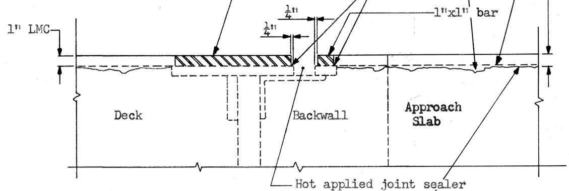
**VERTICAL EXTENSION OF STRUCTURAL EXPANSION JOINTS**
