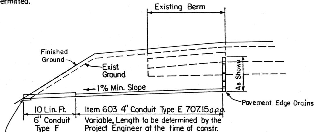
NOTE: For erosion control pad and animal guard see Std. Drwg. MC-4.
