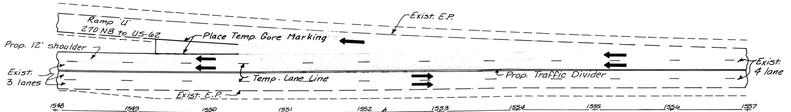
Work Zone Pavement Markings as shown should be in place for the two-way traffic. Replace with appropriate pavement markings when SB traffic is returned to the SB lanes and the final overlay is placed.
