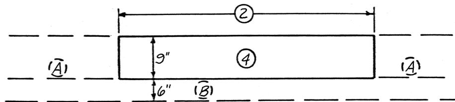
Section AA - Pavement Repair Detail
