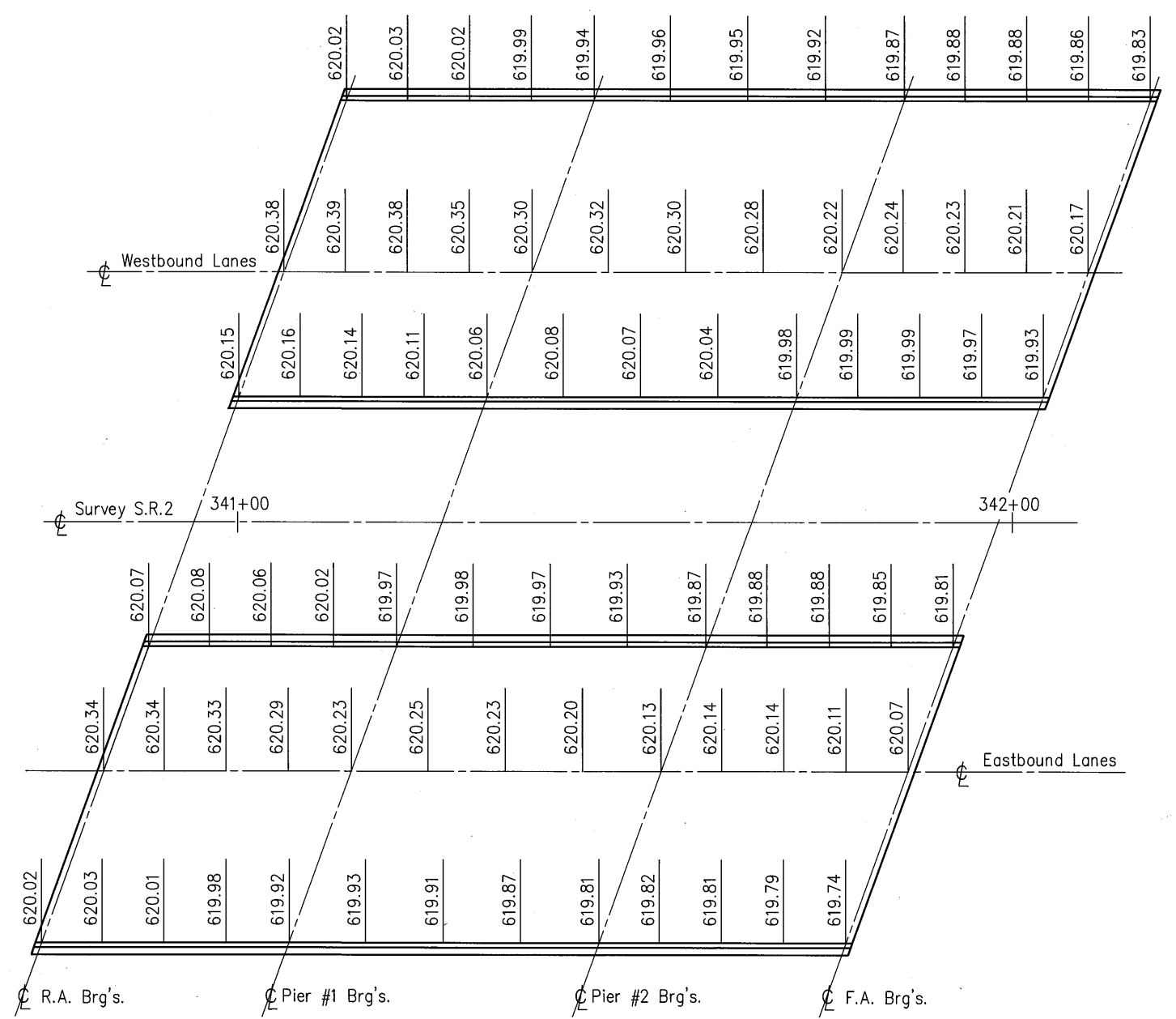
DECK PLAN Screed Elevations Given
