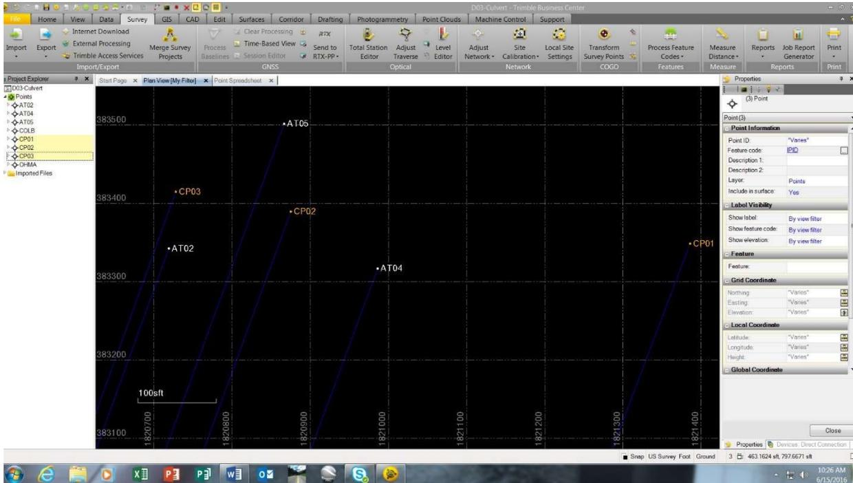
Step 2.) Select points that are to be used to calculate the Project Scale Factor. Points selected should represent a good overall elevation (high, low, mean elevation) of the project.
