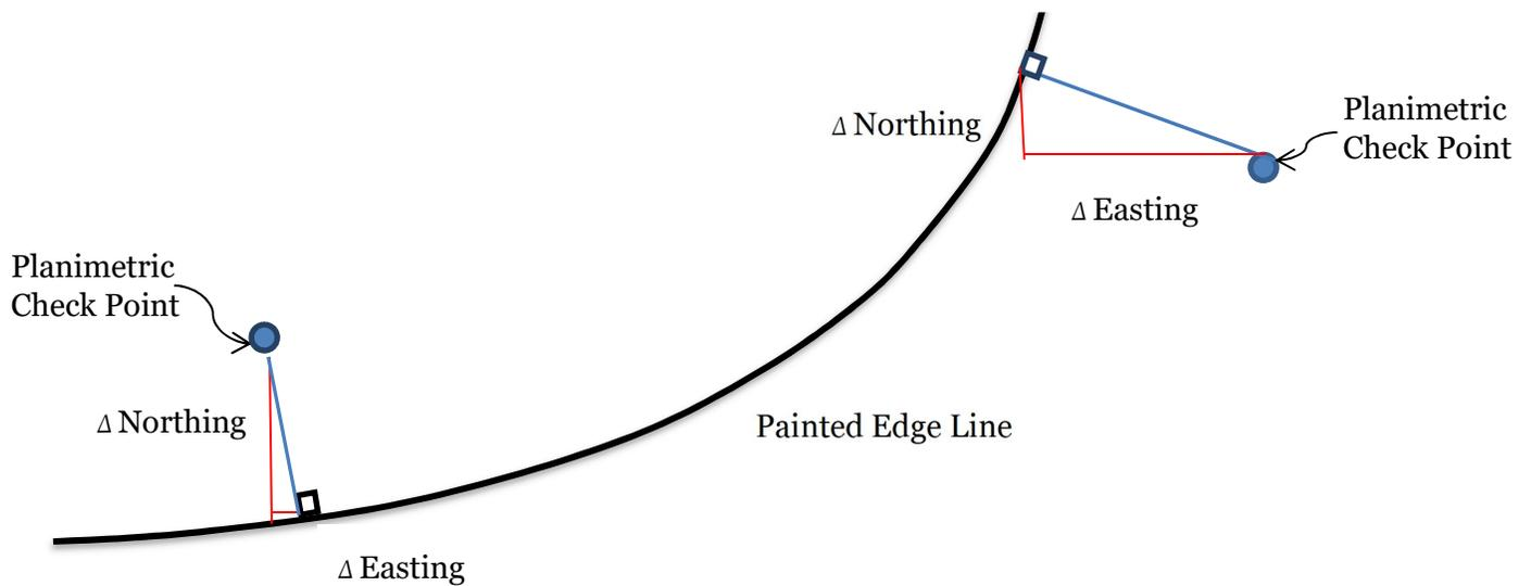
Measurements are taken perpendicular to the center of the painted edge line. Determine the  $\Delta$  Northing and  $\Delta$  Easting components for use in Horizontal Planimetric Feature Accuracy Test.
