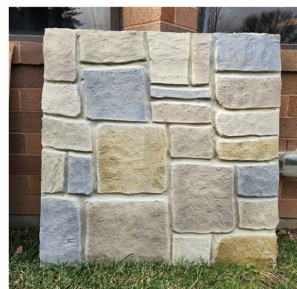
COLOR MOCK UP BASIS OF DESIGN PROVIDED BY CONCRETE ARTISTS (513) 400-0482, OR APPROVED EQUAL. CONTRACTOR TO COORDINATE TEST PANEL COLORS WITH OWNER, ENGINEER AND LANDSCAPE ARCHITECT PRIOR TO CONSTRUCTION.
