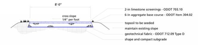
Note: Asphalt Surface is used where trail grade exceeds 4% or where bridle trail is combined with Towpath.
