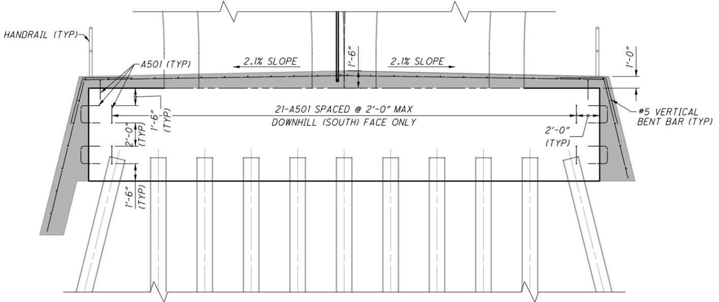
**FOOTING DOWEL FRONT ELEVATION**
