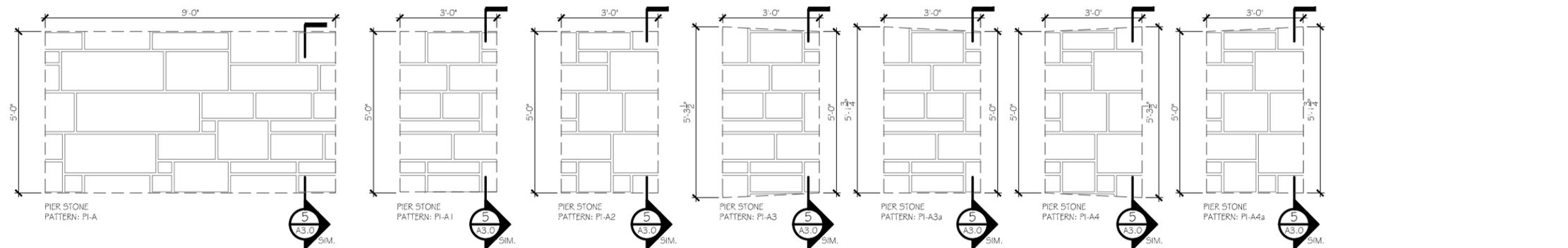
4 ENLARGED ELEVATION: PIER STONE PATTERNS
