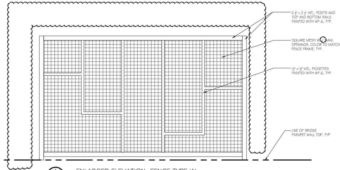
1 ENLARGED ELEVATION: FENCE TYPE 'A'
