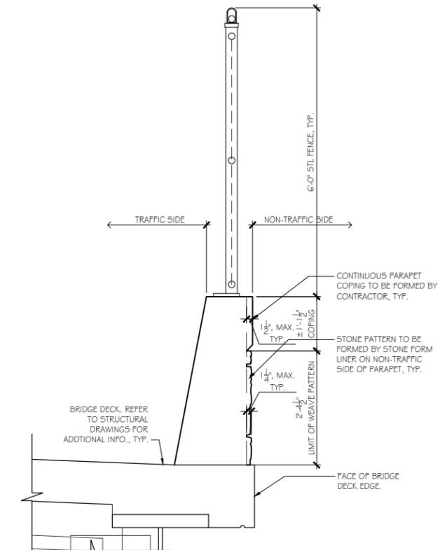
**3** TYPICAL DETAIL: PARAPET WALL @ STONE PATTERN
