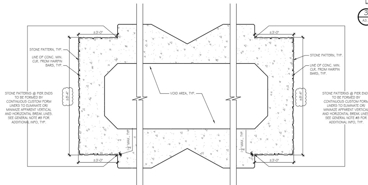
**5** TYPICAL PLAN DETAIL: STONE PATTERN @ PIER END
