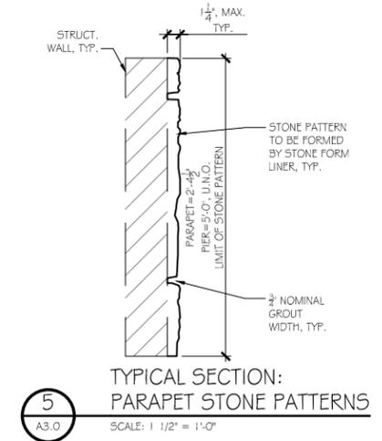
5 TYPICAL SECTION: PARAPET STONE PATTERNS
