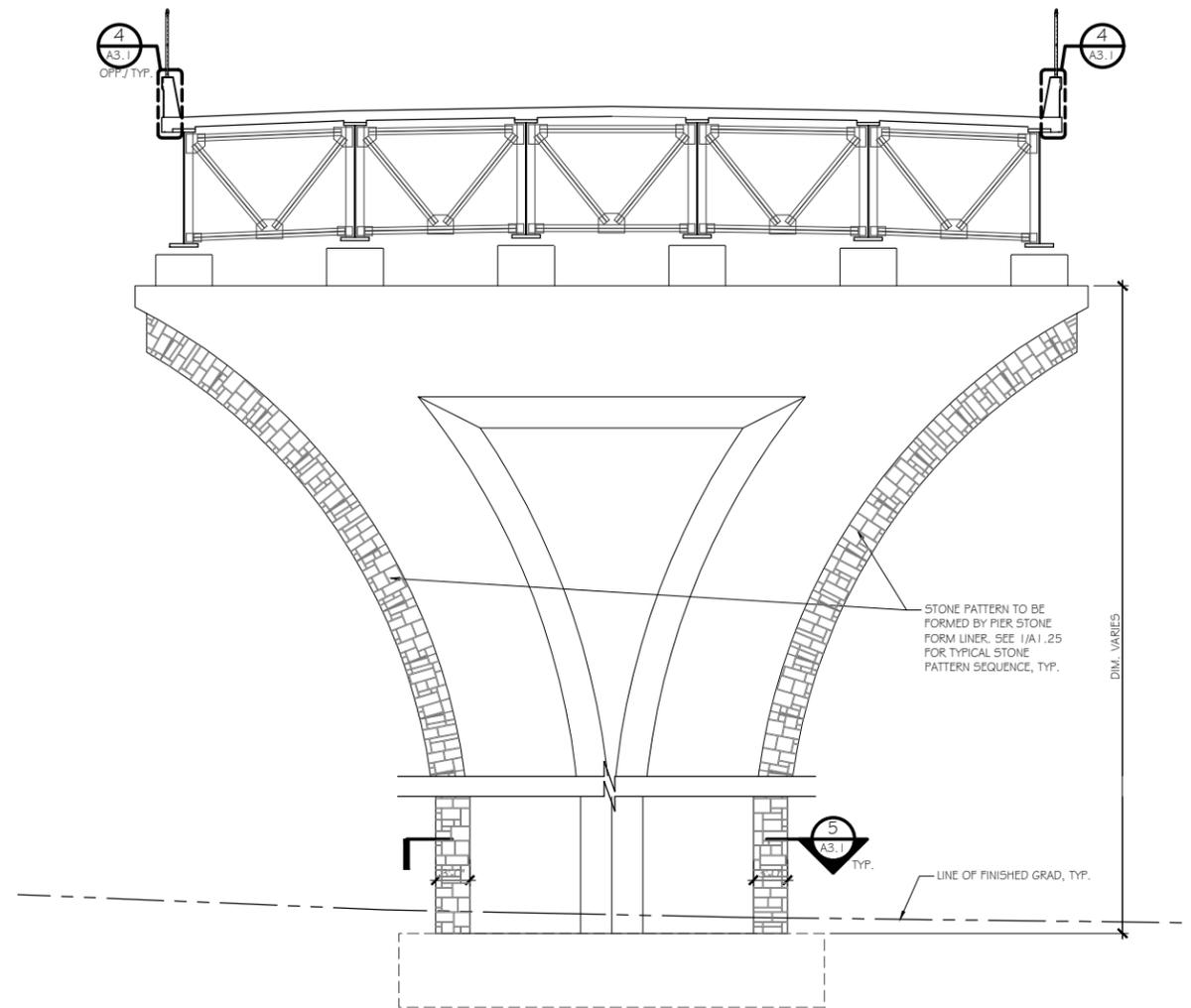
**1** TYPICAL SECTION/ELEVATION: PIER & BRIDGE DECK
