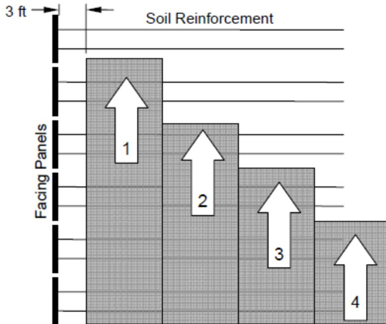
**Figure 840.06-2 Procedure for SGB Placement and Compaction (Plan View)**
