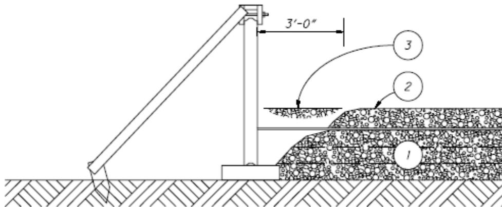
**Figure 840.06-1 Backfilling for the First Row of Panels Only**
