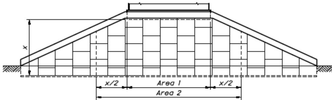
*Use the same soil reinforcement design in Area 2 as that required under the footing (Area 1).*
