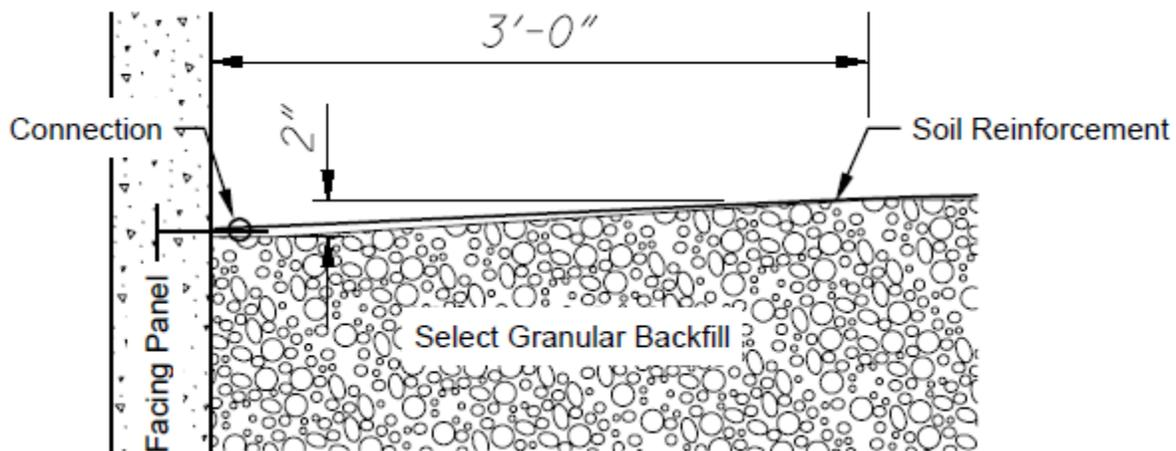
**Figure 840.06-4 SGB at Connection**
