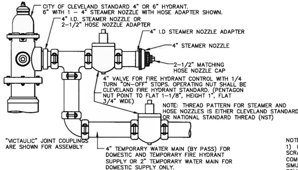
**TEMPORARY WATER MAIN & HYDRANT CONNECTION ASSEMBLY-A TO PROVIDE SIMULTANEOUS SERVICE IN EXISTING HYDRANT AND TEMPORARY BYPASS MAIN (STD-H14)**
