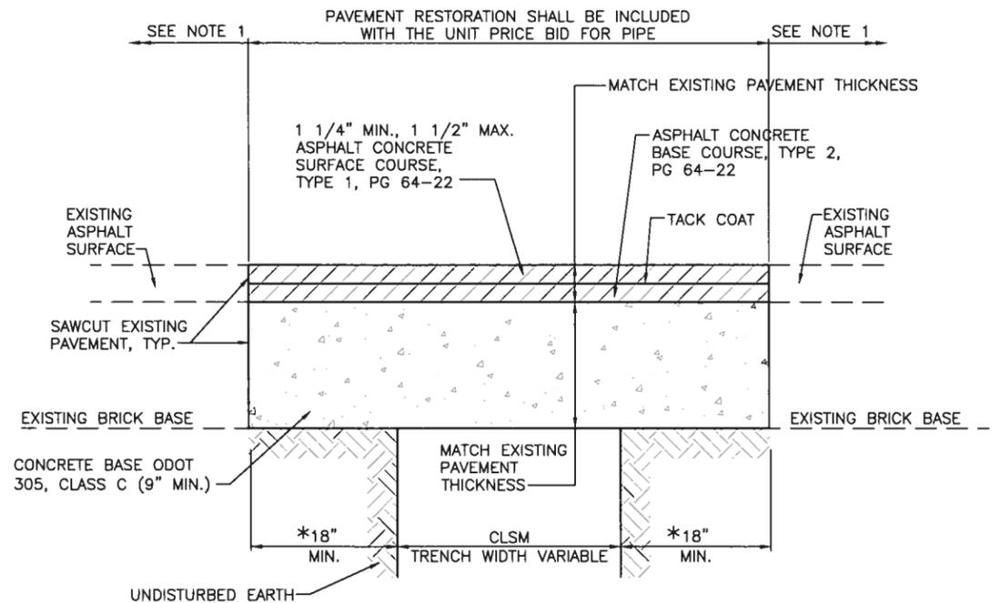
\*CONTINUE PAVEMENT REPLACEMENT TO CURB WHERE SAWCUT OCCURS LESS THAN 3' FROM FACE OF CURB
