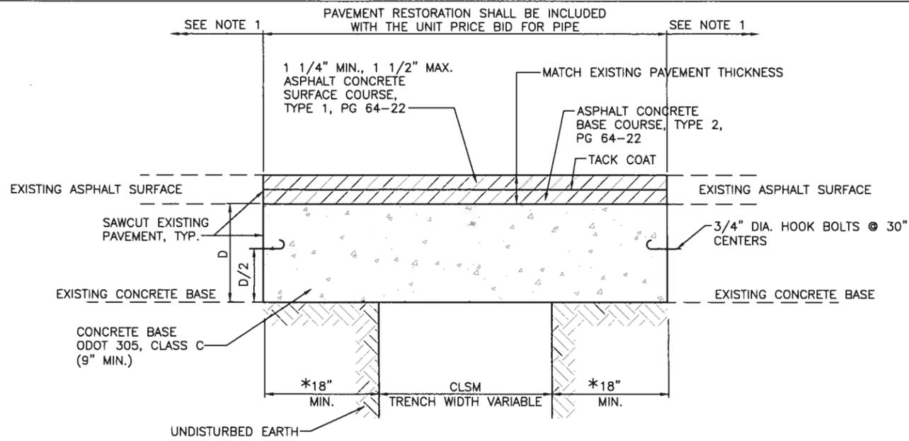
\*CONTINUE PAVEMENT REPLACEMENT TO CURB WHERE SAWCUT OCCURS LESS THAN 3' FROM FACE OF CURB
