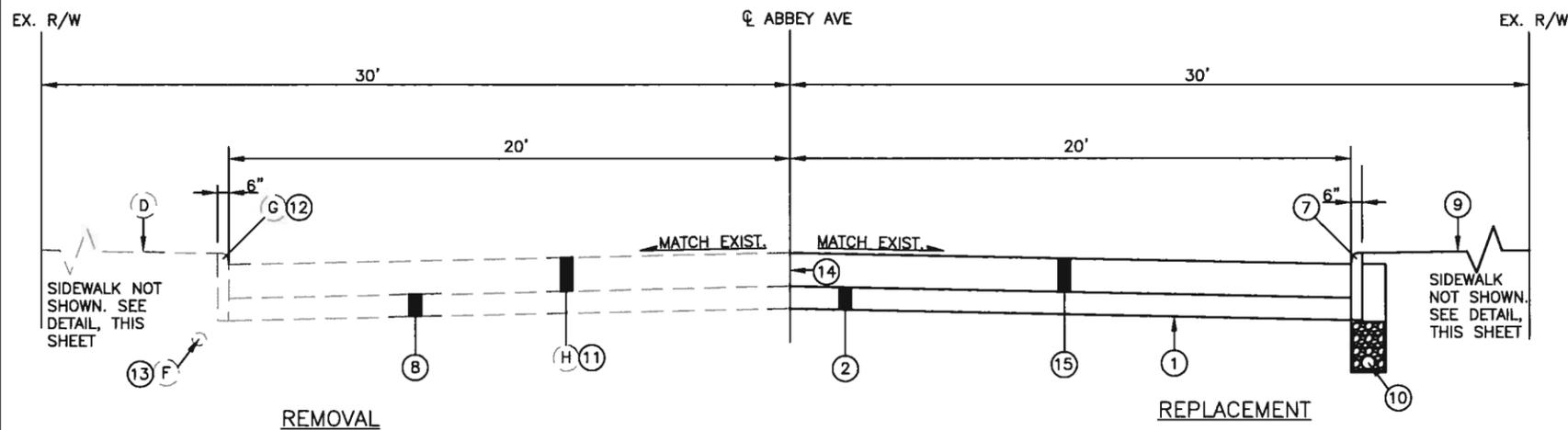
TYPICAL PAVEMENT SECTION-ABBAY AVE AT MANHOLE NO.1 AND NO.2
