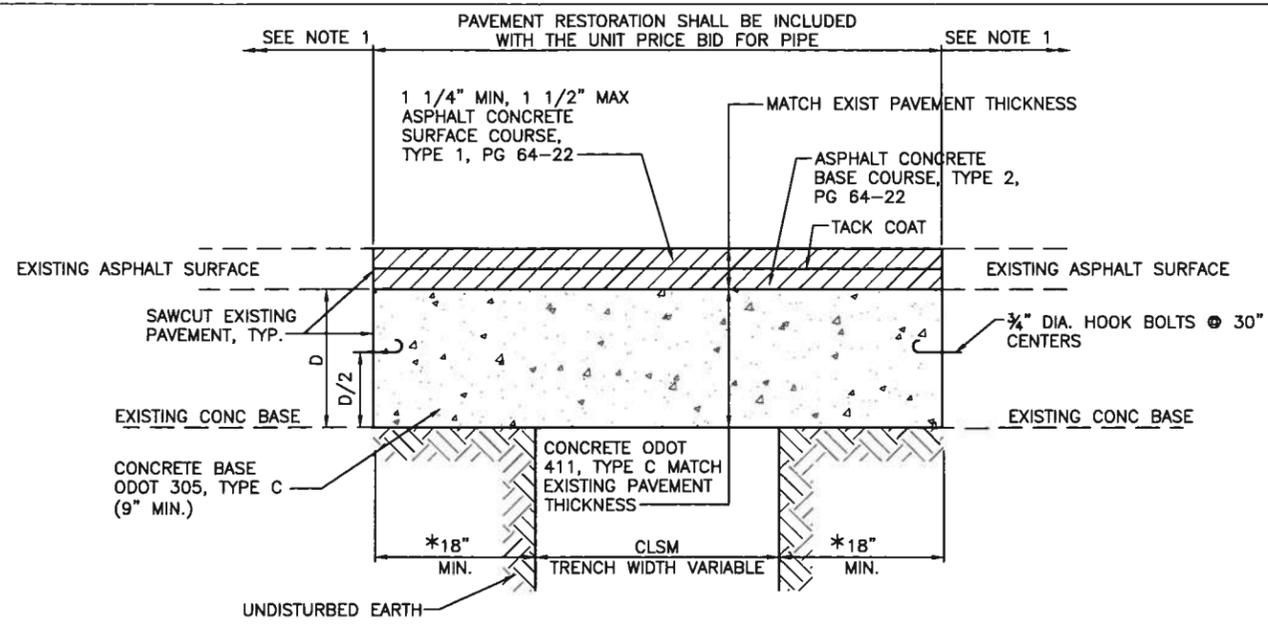
TYPICAL TRENCH DETAIL FOR ASPHALT PAVEMENT WITH CONCRETE BASE
