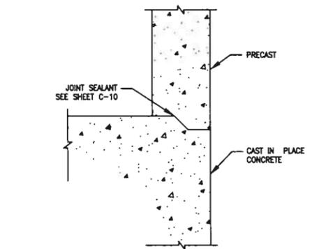
PRECAST RISER TO C.I.P. CONCRETE JOINT DETAIL
