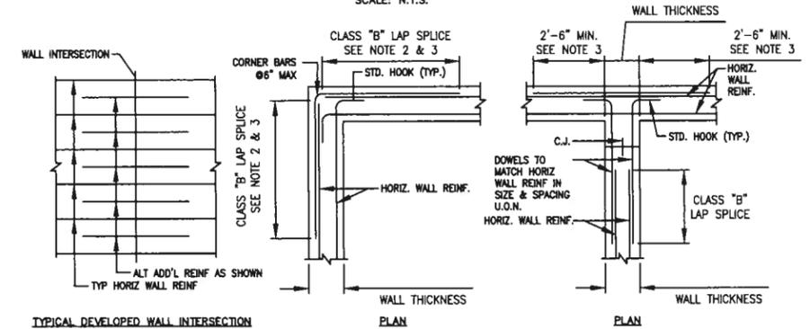
TYPICAL REINFORCEMENT DETAIL AT WALL INTERSECTIONS
