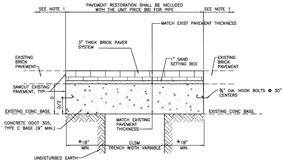
TYPICAL TRENCH DETAIL FOR BRICK PAVEMENT WITH CONCRETE BASE
