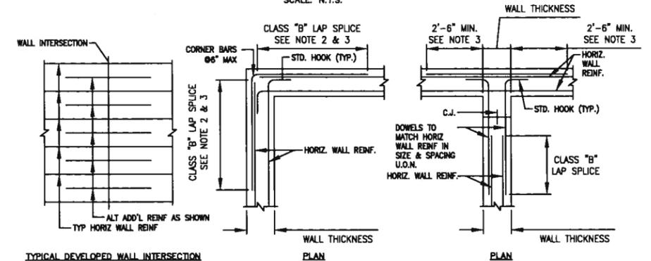
TYPICAL REINFORCEMENT DETAIL AT WALL INTERSECTIONS
