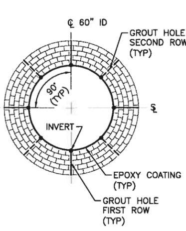
NOTE: GROUT HOLE PATTERN FOR CUT-OFF & CONTACT GROUTING FROM EXISTING INTERCEPTOR.
