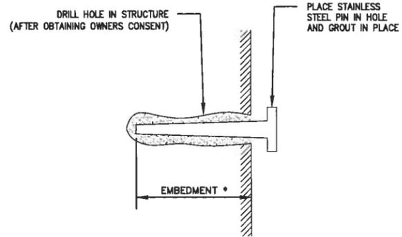
\* EMBED TO A DEPTH AS NECESSARY TO PROVIDE A RIGID IMMOVABLE POINT
