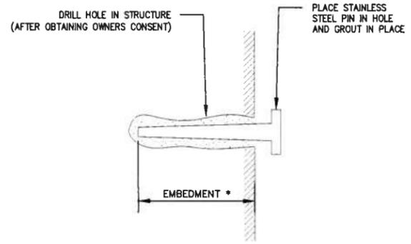
\* EMBED TO A DEPTH AS NECESSARY TO PROVIDE A RIGID IMMOVABLE POINT
