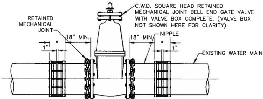
NOTE: BEFORE CUTTING EXISTING WATER MAIN, THE NIPPLES SHALL BE CONNECTED TO THE MECHANICAL JOINT BELL END GATE VALVE. AFTER CUTTING PIPE, FINAL CONNECTIONS SHALL BE MADE WITH COUPLINGS/SOLID SLEEVES AS SPECIFIED.
