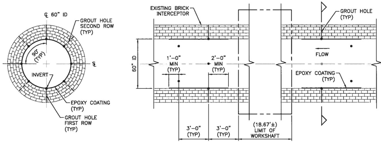
NOTE: GROUT HOLE PATTERN FOR CUT-OFF & CONTACT GROUTING FROM EXISTING INTERCEPTOR.
