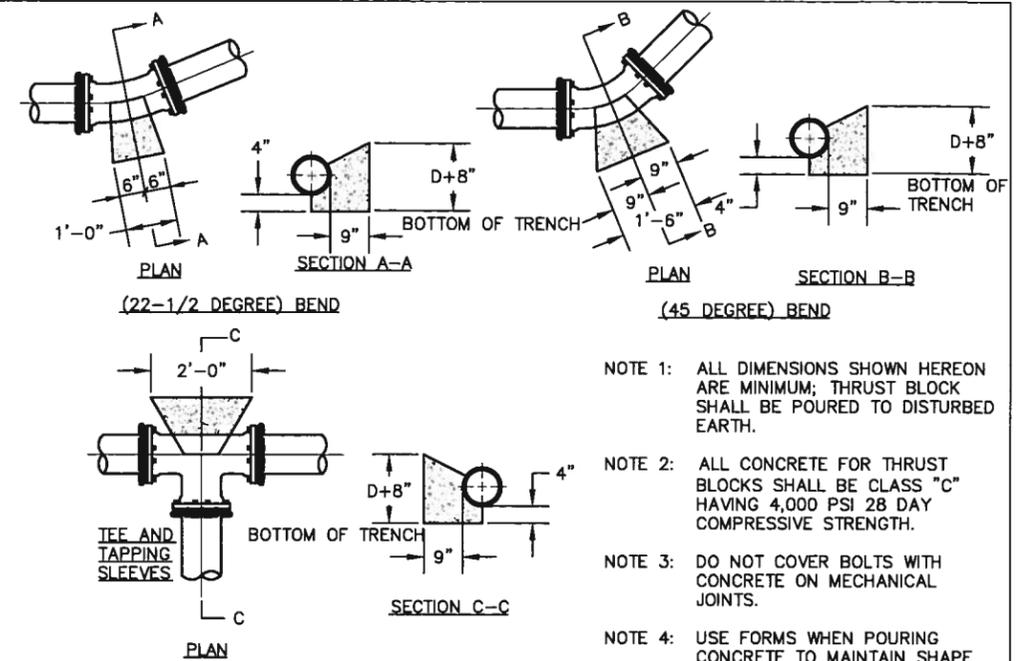
**TYPICAL THRUST BLOCK DETAIL FOR HORIZONTAL DEFLECTION FOR PIPE UP TO 16" DIAMETER (STD-006)**
