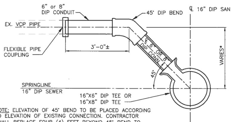
\*NOTE: ELEVATION OF 45° BEND TO BE PLACED ACCORDING TO ELEVATION OF EXISTING CONNECTION. CONTRACTOR SHALL REPLACE FOUR (4) FEET BEYOND 45° BEND TO CONNECT TO THE EXISTING PIPE.
