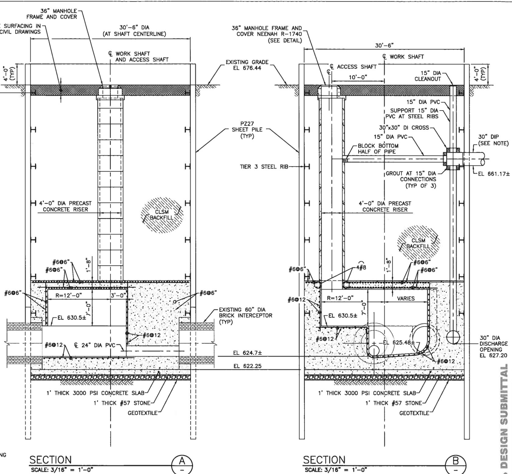
NOTE: BEFORE INSTALLING 30" DIP AND 30"x30" CROSS, BACKFILL SHAFT TO 2 FT BELOW TIER 3 STEEL RIB. THEN REMOVE TIER 3 STEEL RIB AND INSTALL DI PIPING.
