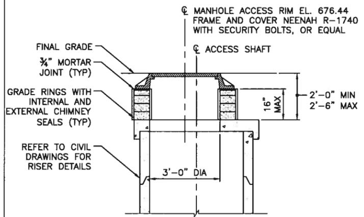
**FRAME AND COVER 36" MANHOLE DETAIL**
