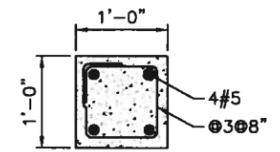
**REINFORCEMENT BEAM DETAIL**
