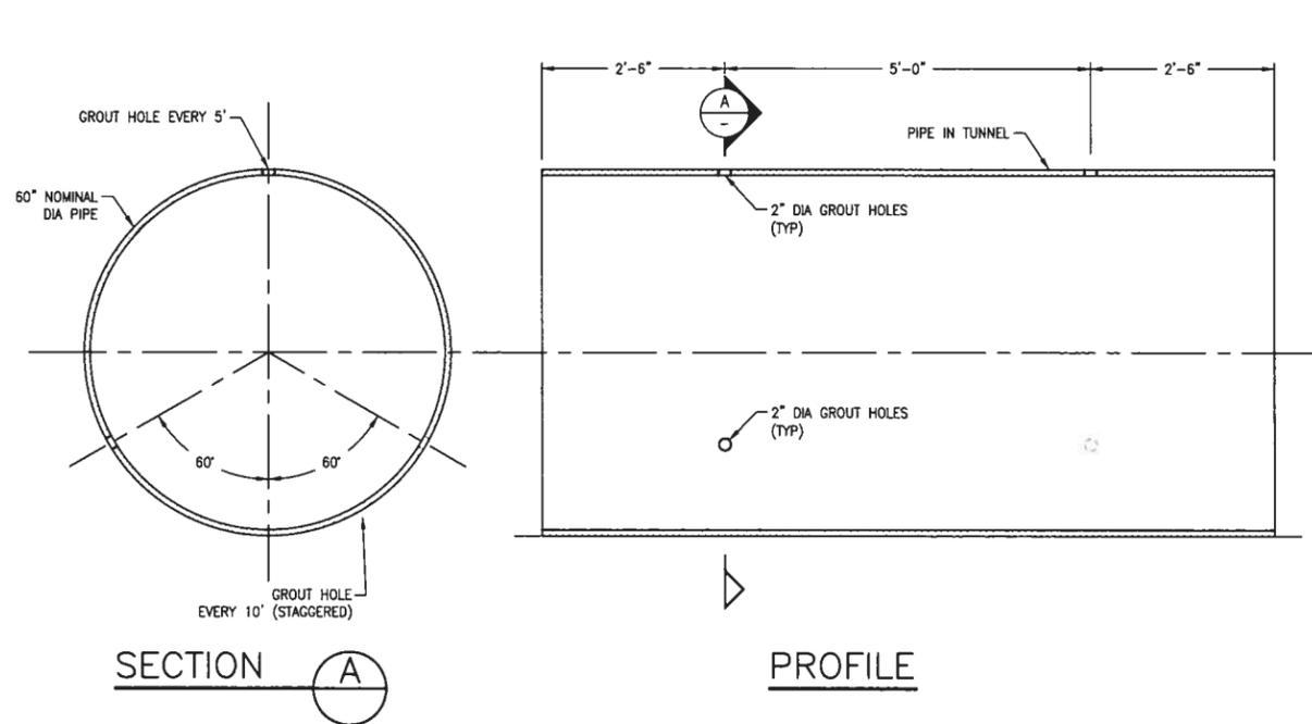
**MICROTUNNEL GROUT HOLE DETAILS**
