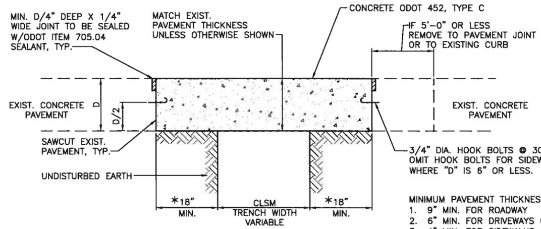
TYPICAL TRENCH DETAIL FOR CONCRETE PAVEMENT
