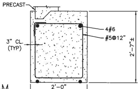
**BEAM REINFORCEMENT DETAIL**
