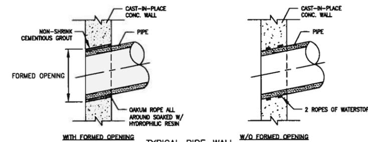
TYPICAL PIPE-WALL PENETRATION DETAIL WITH WATERSTOP
