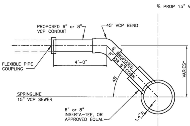
\* NOTE: ELEVATION OF 45° BEND TO BE PLACED ACCORDING TO ELEVATION OF EXISTING CONNECTION. CONTRACTOR SHALL REPLACE FOUR (4) FEET BEYOND 45° BEND TO CONNECT TO THE EXISTING PIPE.
