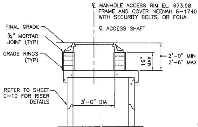
**FRAME AND COVER 36" MANHOLE DETAIL**
