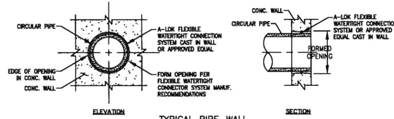
TYPICAL PIPE-WALL PENETRATION DETAIL WITH A-LOK
