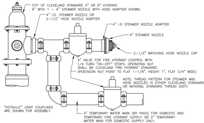
**TEMPORARY WATER MAIN & HYDRANT CONNECTION ASSEMBLY-A TO PROVIDE SIMULTANEOUS SERVICE IN EXISTING HYDRANT AND TEMPORARY BYPASS MAIN (STD-H14)**
