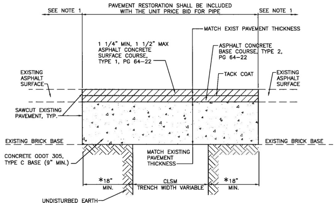
TYPICAL TRENCH DETAIL FOR ASPHALT PAVEMENT WITH BRICK BASE
