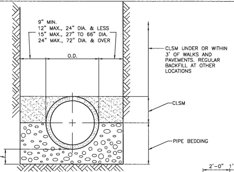
TYPICAL SEWER TRENCH FOR VCP SANITARY SEWER
