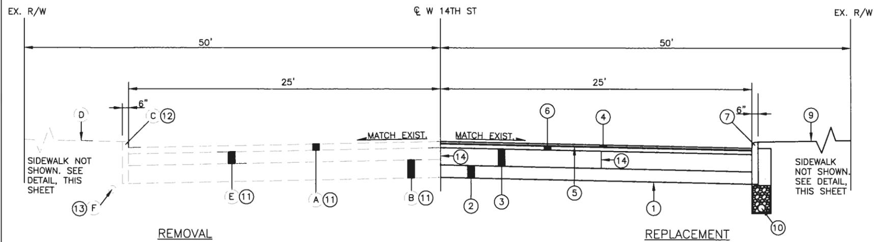
TYPICAL PAVEMENT SECTION-W 14TH ST AT JUNCTION CHAMBER NO.1
