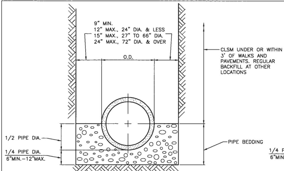
TYPICAL SEWER TRENCH FOR RCP STORM AND SANITARY AND VCP STORM SEWER
