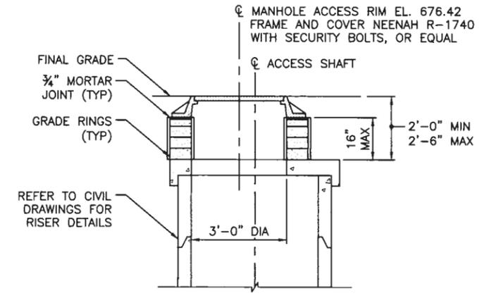
**FRAME AND COVER 36" MANHOLE DETAIL**
