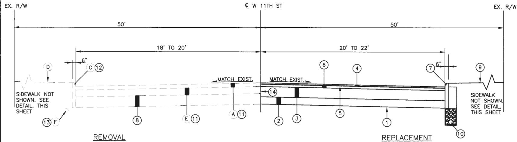
TYPICAL PAVEMENT SECTION-W 11TH ST AT MANHOLE NO.2 AND JUNCTION CHAMBER NO.2
