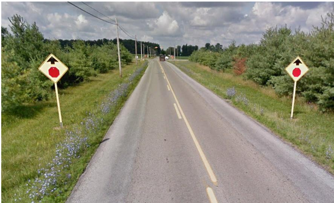
Figure 4: Westbound Ft Amanda Rd - Dual, LED Enhanced Stop Ahead Signs
