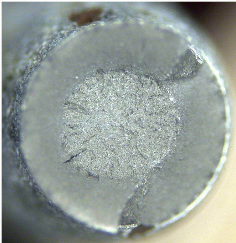
Fig. 22 Wire 2-4 surface (top) and fracture surface after tensile testing (bottom).
