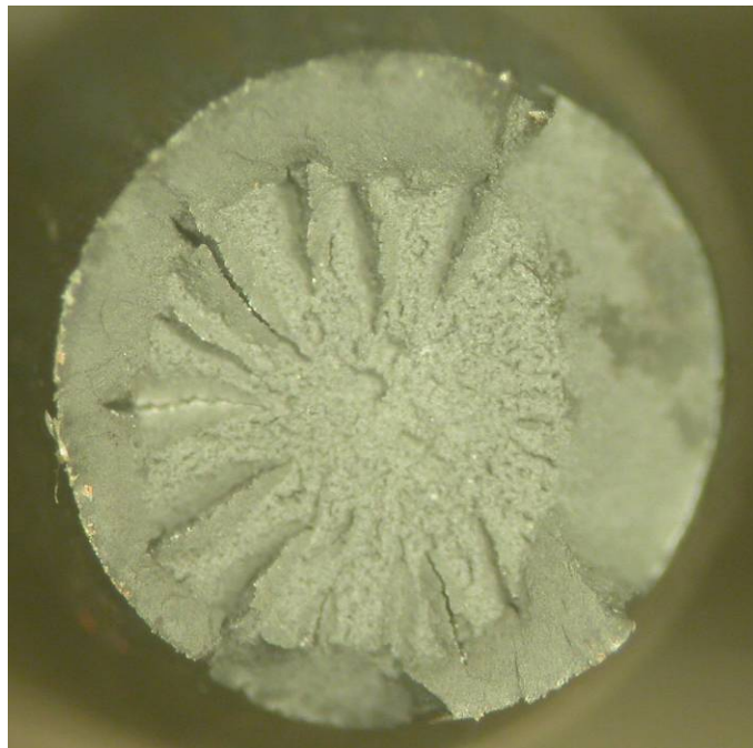
Fig. 76 Wire 10-10 surface (top) and fracture surface after tensile testing (bottom).
