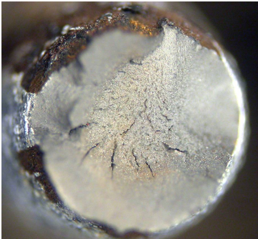
Fig. 27 Wire 3-4 surface (top) and fracture surface after tensile testing (bottom).
