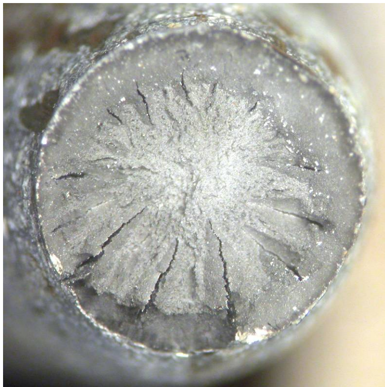
Fig. 90 Wire 12-7 surface (top) and fracture surface after tensile testing (bottom).
