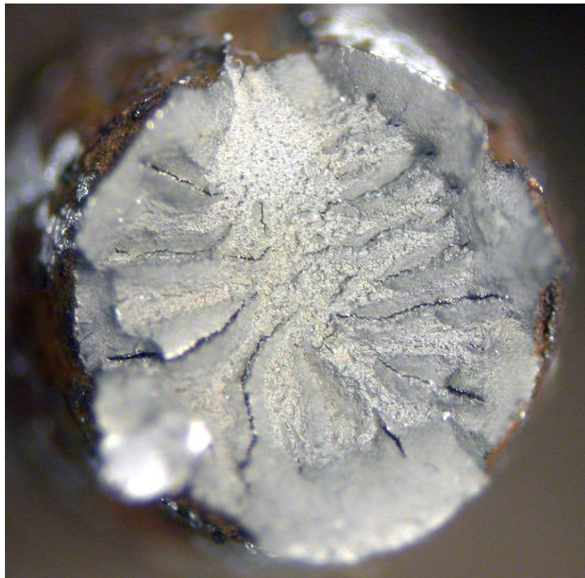
Fig. 31 Wire 4-2 surface (top) and fracture surface after tensile testing (bottom).
