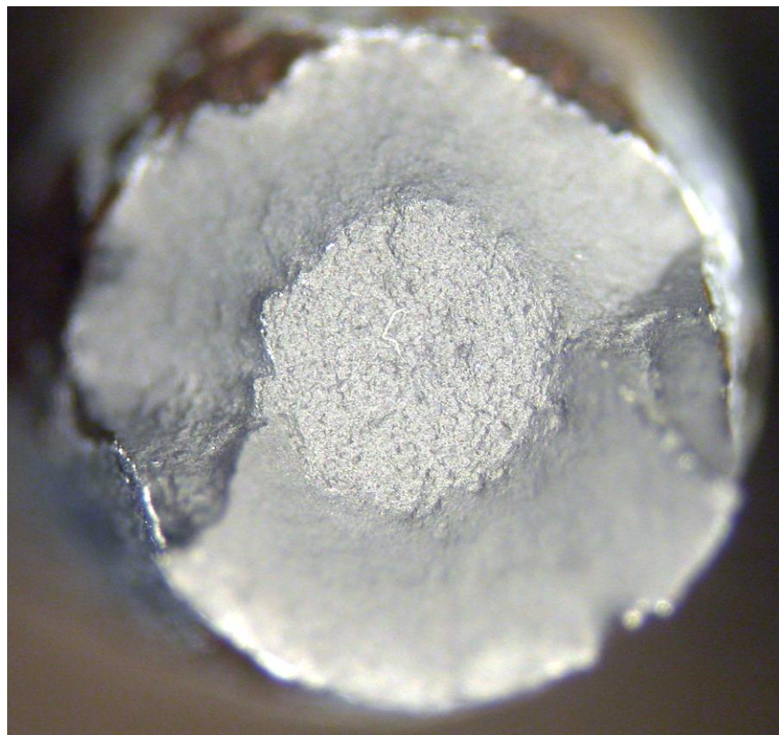
Fig. 50 Wire 7-2 surface (top) and fracture surface after tensile testing (bottom).
