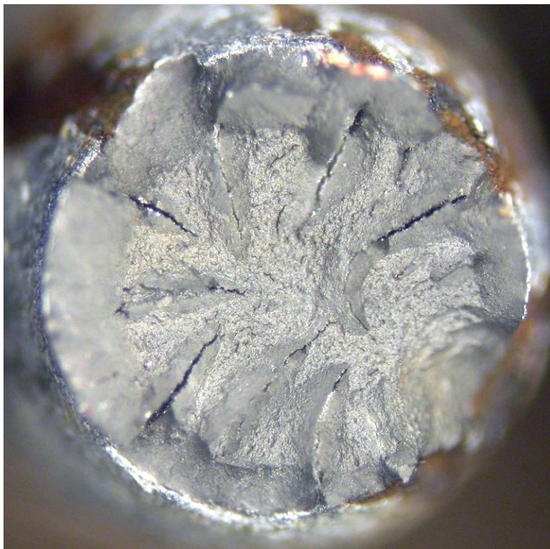
Fig. 45 Wire 6-2 surface (top) and fracture surface after tensile testing (bottom).
