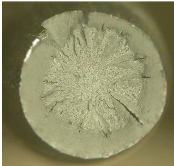
Fig. 74 Wire 10-8 surface (top) and fracture surface after tensile testing (bottom).
