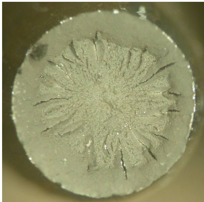
Fig. 95 Wire 13-5 surface (top) and fracture surface after tensile testing (bottom).
