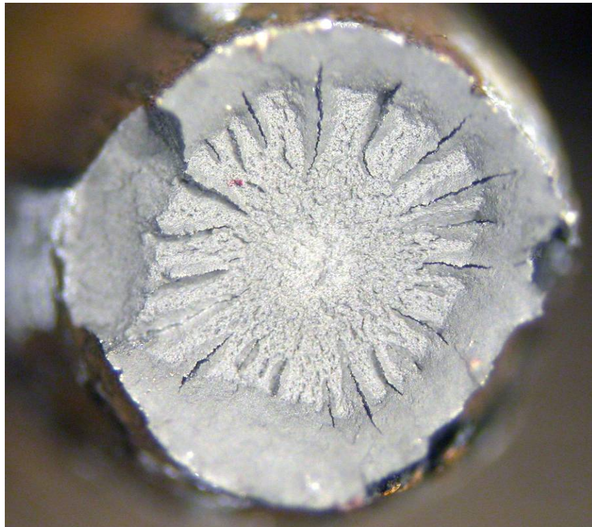
Fig. 41 Wire 5-6 surface (top) and fracture surface after tensile testing (bottom).
