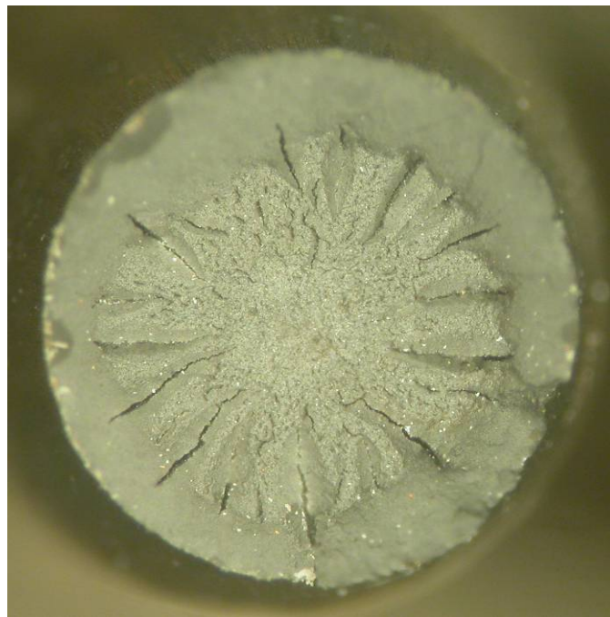
Fig. 93 Wire 13-3 surface (top) and fracture surface after tensile testing (bottom).
