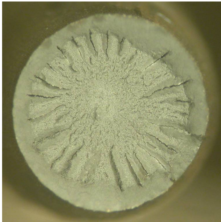
Fig. 82 Wire 11-5 surface (top) and fracture surface after tensile testing (bottom).
