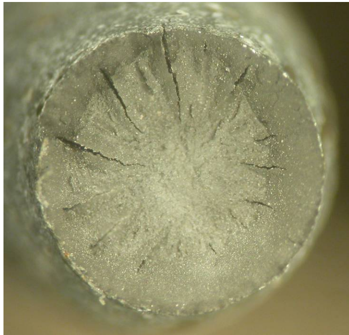
Fig. 89 Wire 12-6 surface (top) and fracture surface after tensile testing (bottom).
