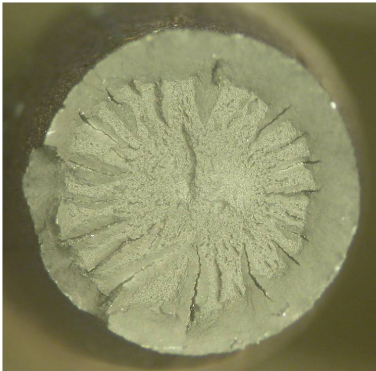
Fig. 78 Wire 11-1 surface (top) and fracture surface after tensile testing (bottom).
