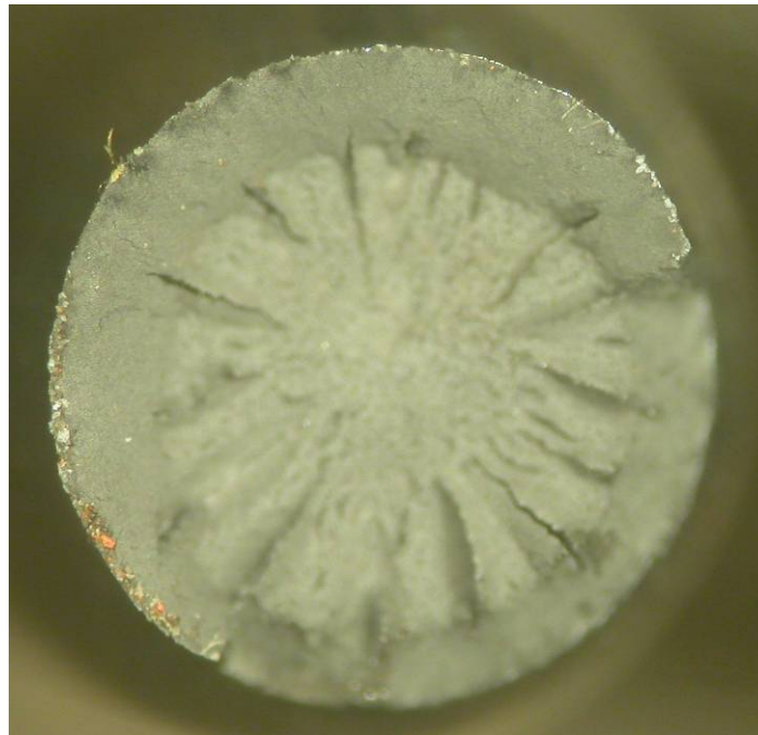
Fig. 71 Wire 10-5 surface (top) and fracture surface after tensile testing (bottom).
