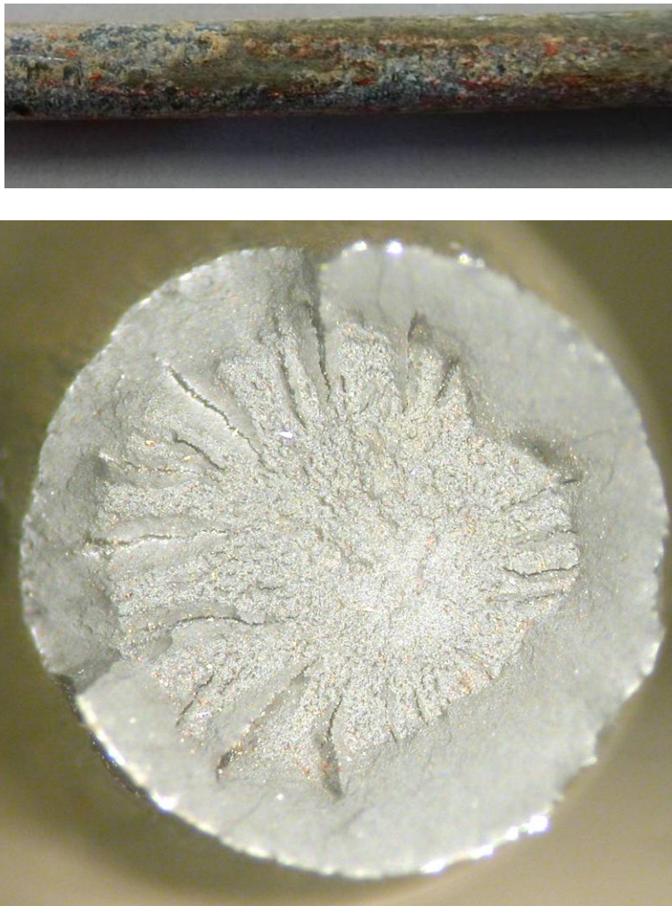
Fig. 61 Wire 9-1 surface (top) and fracture surface after tensile testing (bottom).
