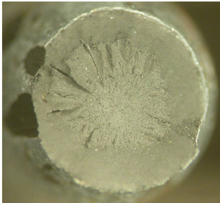
Fig. 64 Wire 9-4 surface (top) and fracture surface after tensile testing (bottom).
