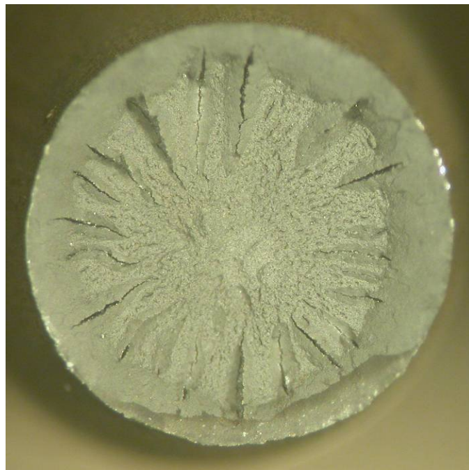
Fig. 80 Wire 11-3 surface (top) and fracture surface after tensile testing (bottom).
