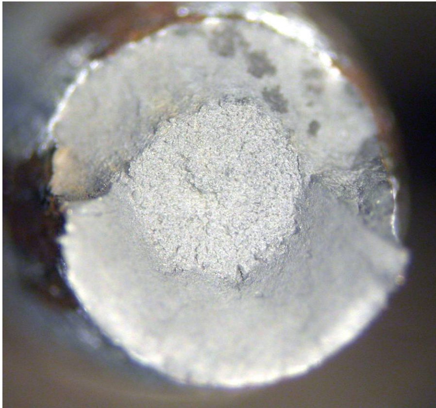
Fig. 25 Wire 3-2 surface (top) and fracture surface after tensile testing (bottom).
