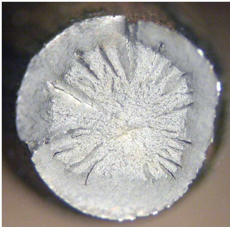
Fig. 28 Wire 3-5 surface (top) and fracture surface after tensile testing (bottom).
