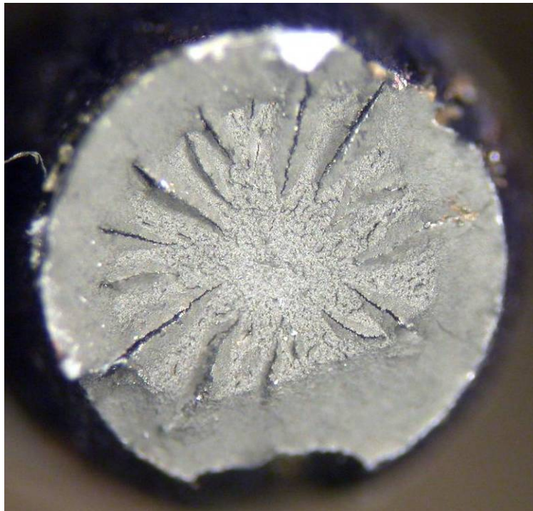
Fig. 44 Wire 6-1 surface (top) and fracture surface after tensile testing (bottom).
