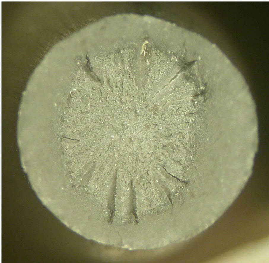
Fig. 68 Wire 10-2 surface (top) and fracture surface after tensile testing (bottom).
