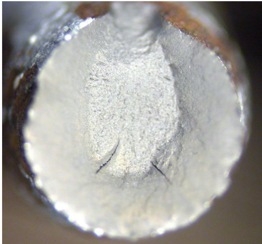
Fig. 48 Wire 6-5 surface (top) and fracture surface after tensile testing (bottom).
