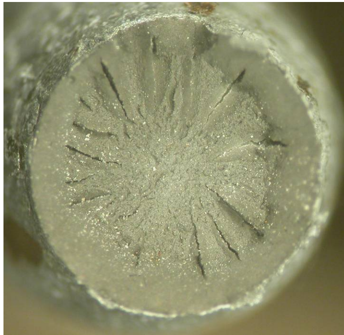
Fig. 88 Wire 12-5 surface (top) and fracture surface after tensile testing (bottom).
