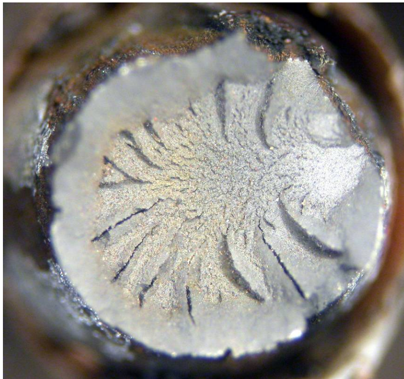
Fig. 38 Wire 5-3 surface (top) and fracture surface after tensile testing (bottom).
