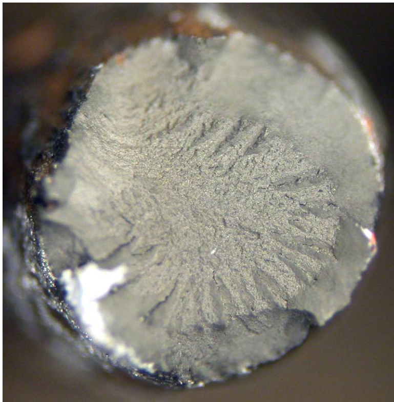
Fig. 43 Wire 5-8 surface (top) and fracture surface after tensile testing (bottom).
