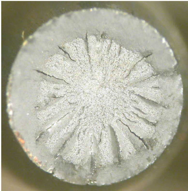
Fig. 72 Wire 10-6 surface (top) and fracture surface after tensile testing (bottom).
