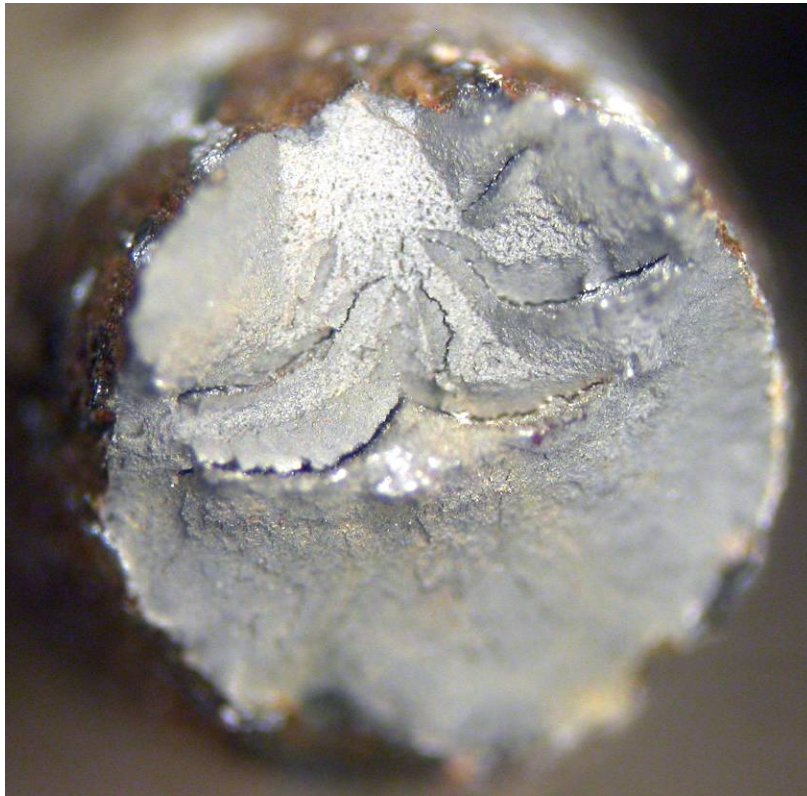
Fig. 34 Wire 4-5 surface (top) and fracture surface after tensile testing (bottom).
