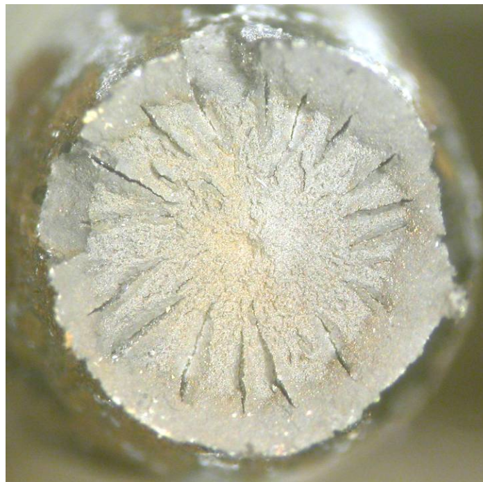
Fig. 56 Wire 8-2 surface (top) and fracture surface after tensile testing (bottom).
