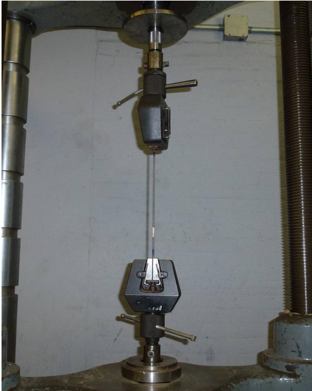
Fig. 11 General view of a wire during the tensile test.
