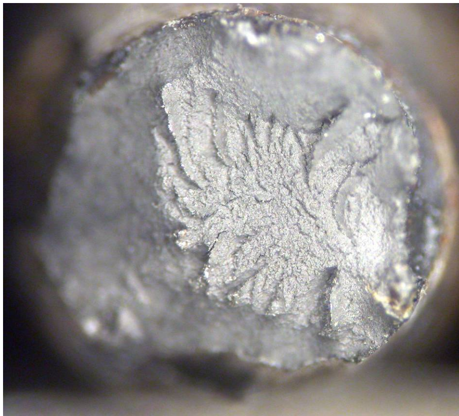
Fig. 53 Wire 7-5 surface (top) and fracture surface after tensile testing (bottom).
