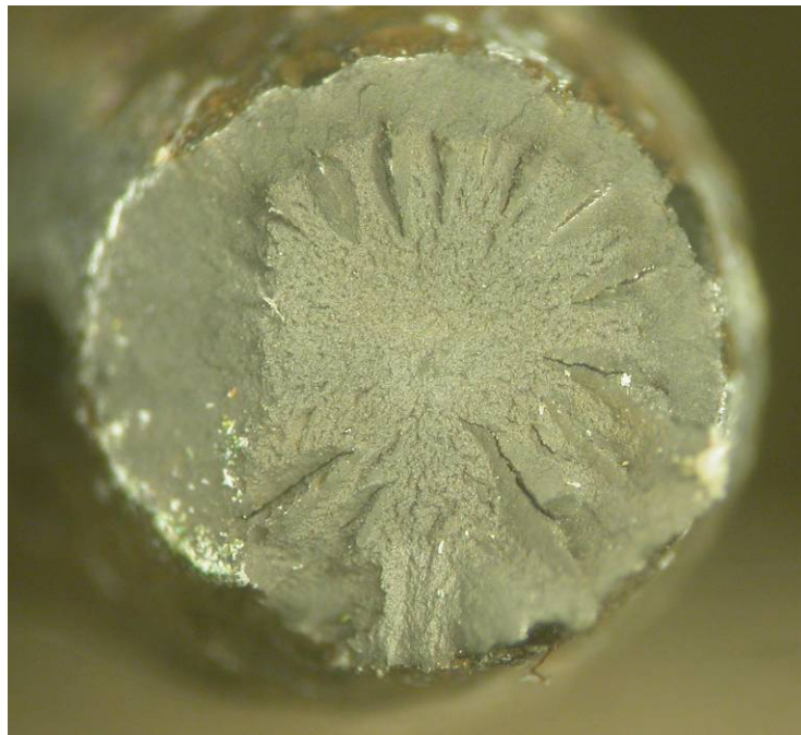
Fig. 57 Wire 8-3 surface (top) and fracture surface after tensile testing (bottom).
