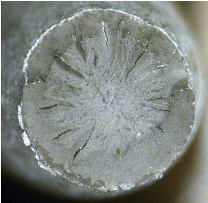
Fig. 86 Wire 12-3 surface (top) and fracture surface after tensile testing (bottom).
