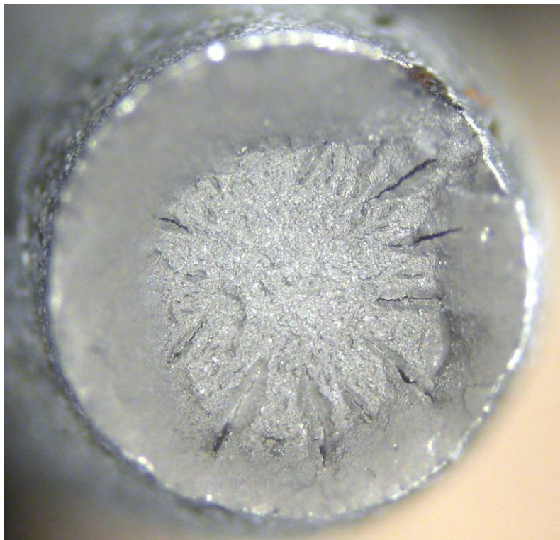
Fig. 23 Wire 2-5 surface (top) and fracture surface after tensile testing (bottom).
