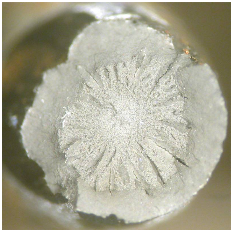
Fig. 54 Wire 7-6 surface (top) and fracture surface after tensile testing (bottom).
