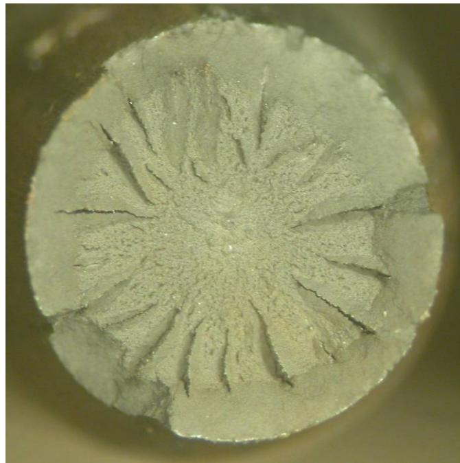
Fig. 81 Wire 11-4 surface (top) and fracture surface after tensile testing (bottom).
