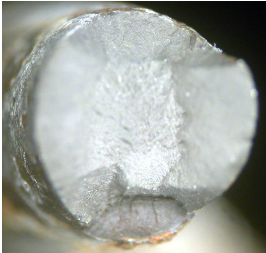
Fig. 26 Wire 3-3 surface (top) and fracture surface after tensile testing (bottom).
