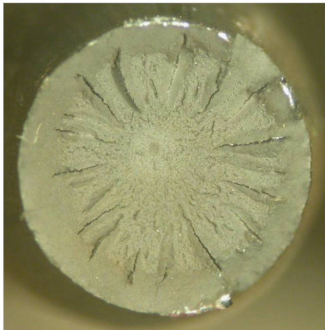
Fig. 79 Wire 11-2 surface (top) and fracture surface after tensile testing (bottom).
