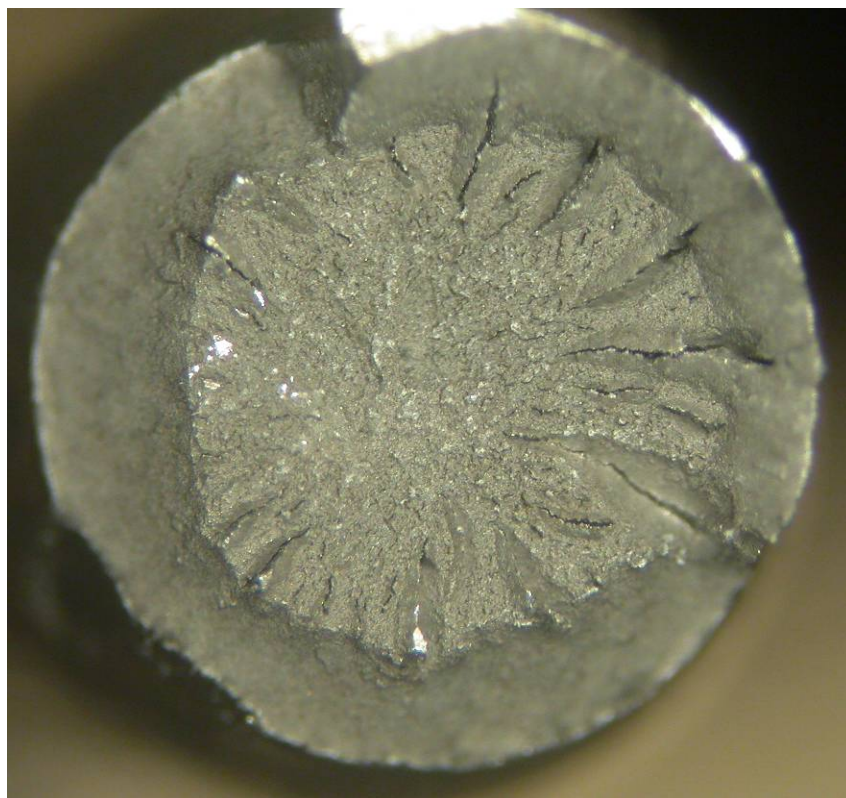
Fig. 62 Wire 9-2 surface (top) and fracture surface after tensile testing (bottom).
