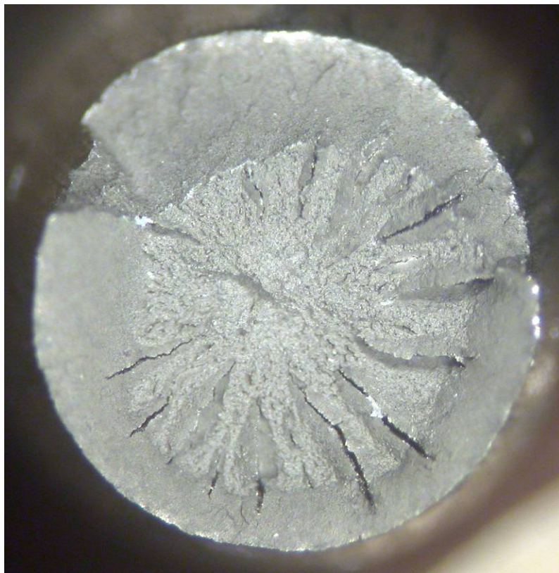
Fig. 73 Wire 10-7 surface (top) and fracture surface after tensile testing (bottom).
