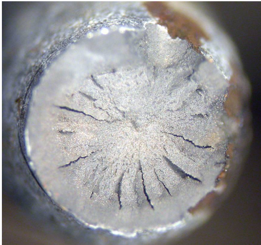
Fig. 46 Wire 6-3 surface (top) and fracture surface after tensile testing (bottom).
