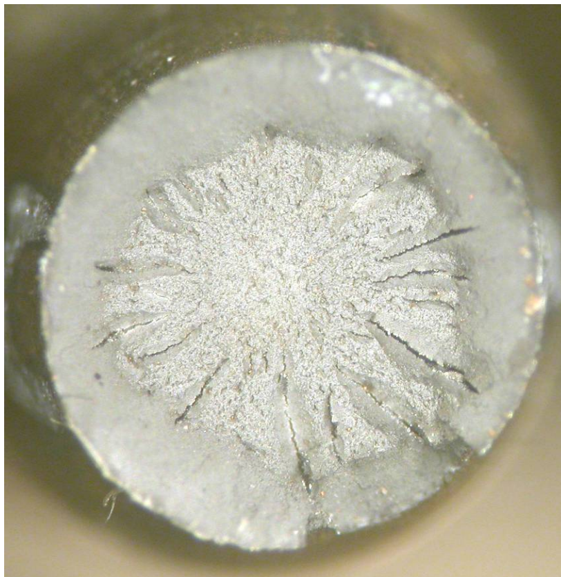
Fig. 69 Wire 10-3 surface (top) and fracture surface after tensile testing (bottom).
