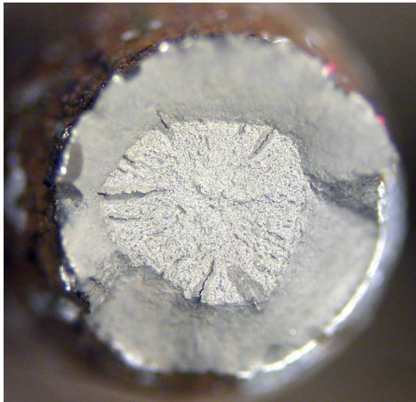
Fig. 24 Wire 3-1 surface (top) and fracture surface after tensile testing (bottom).
