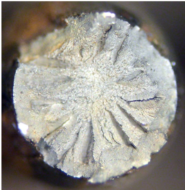
Fig. 33 Wire 4-4 surface (top) and fracture surface after tensile testing (bottom).
