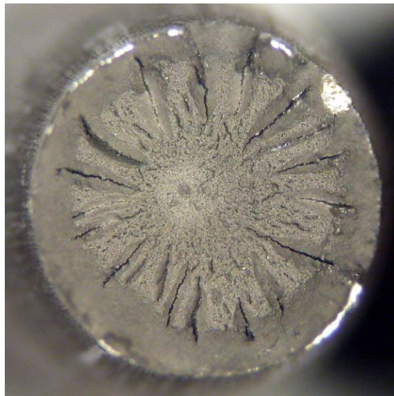
Fig. 114 Wire 11-2 fracture profile (top) and fracture surfaces (bottom).
