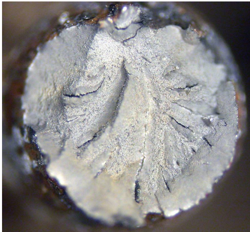
Fig. 32 Wire 4-3 surface (top) and fracture surface after tensile testing (bottom).
