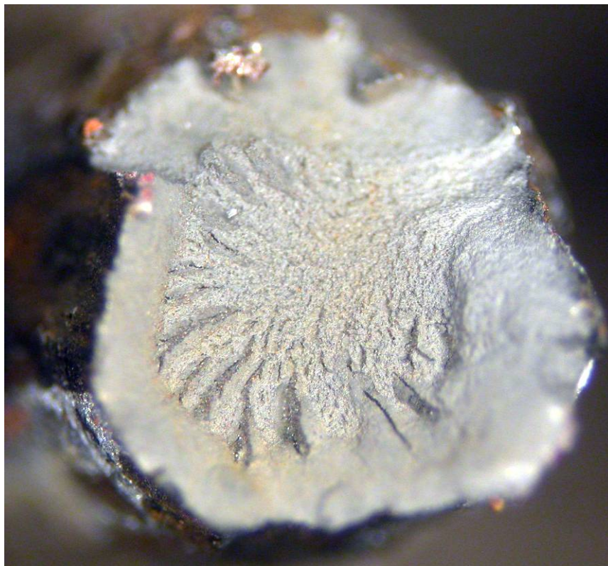
Fig. 37 Wire 5-2 surface (top) and fracture surface after tensile testing (bottom).
