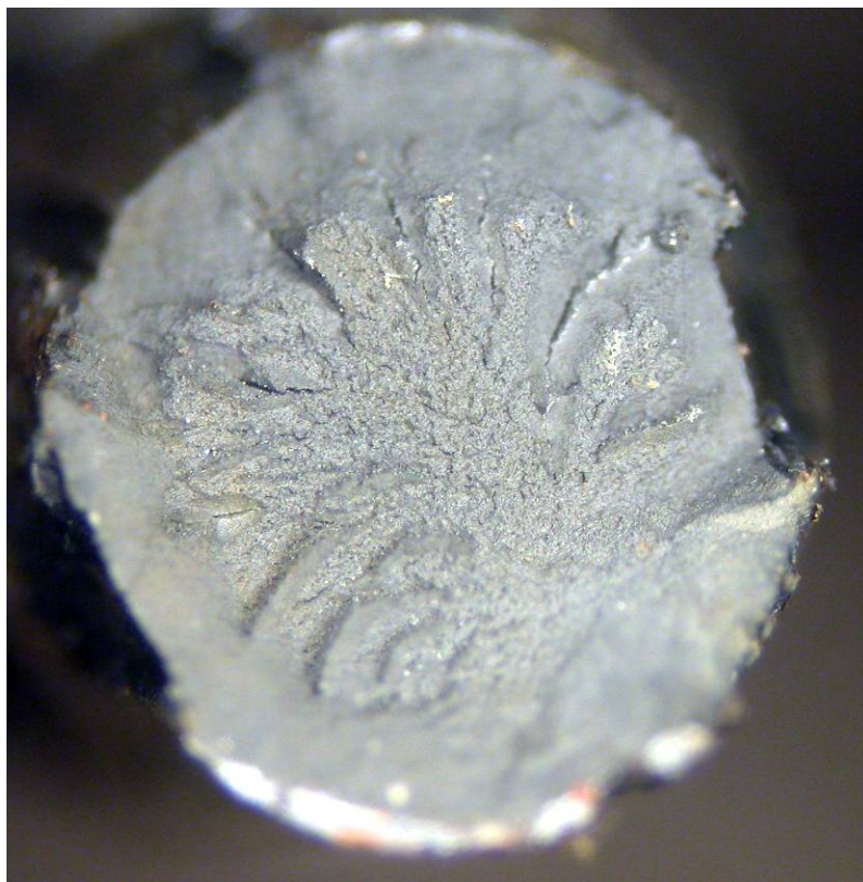
Fig. 40 Wire 5-5 surface (top) and fracture surface after tensile testing (bottom).
