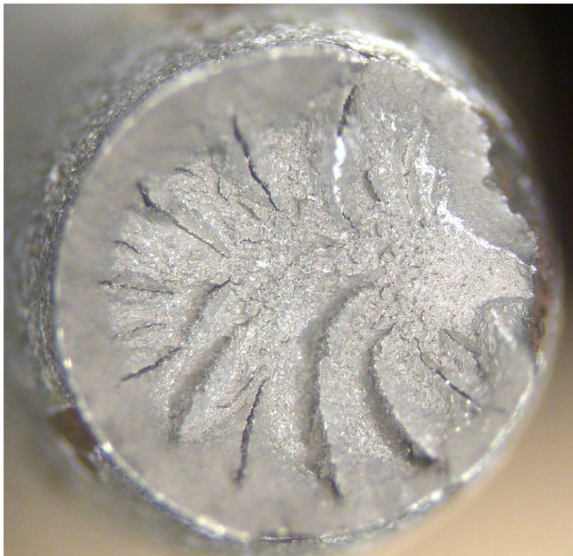
Fig.18 Wire 1-6 surface (top) and fracture surface after tensile testing (bottom).
