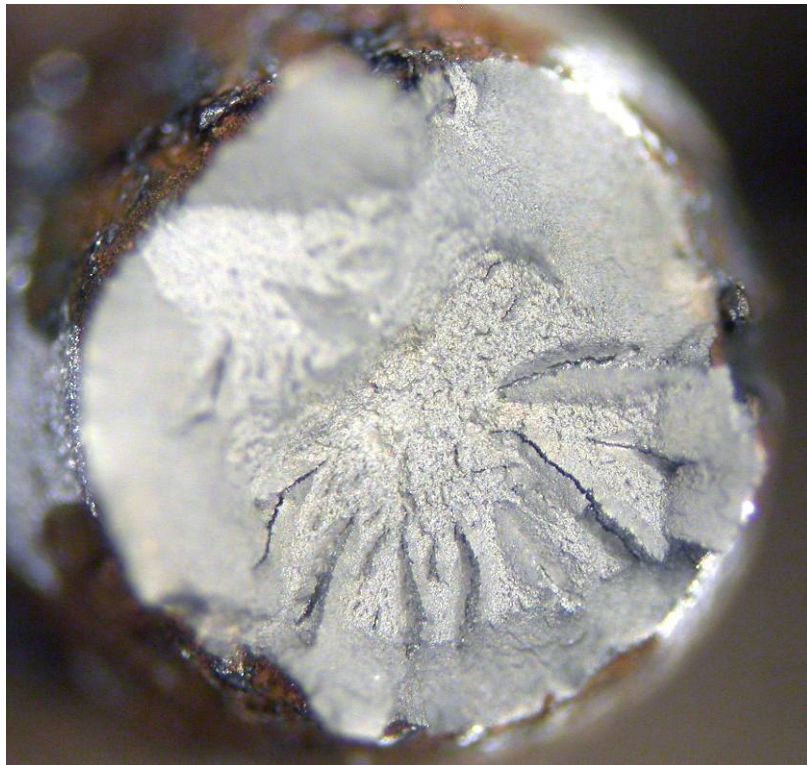
Fig. 35 Wire 4-6 surface (top) and fracture surface after tensile testing (bottom).
