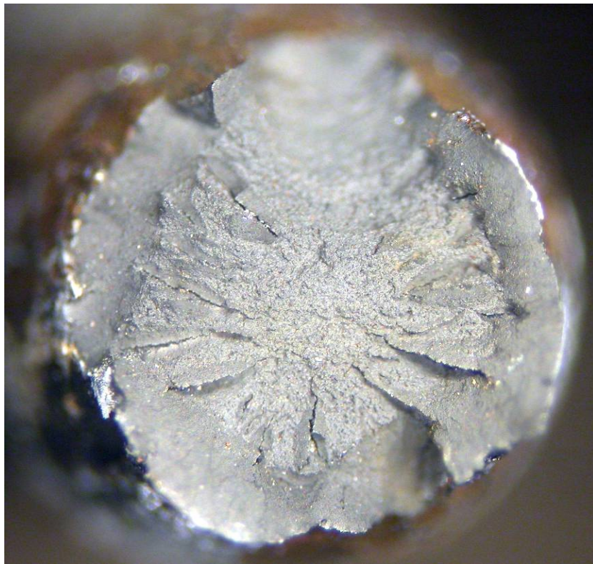
Fig. 30 Wire 4-1 surface (top) and fracture surface after tensile testing (bottom).
