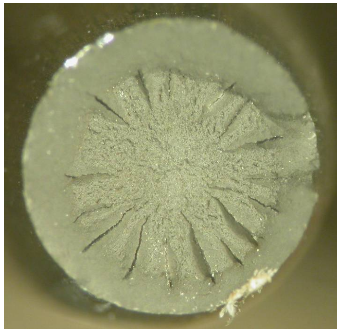
Fig. 92 Wire 13-2 surface (top) and fracture surface after tensile testing (bottom).
