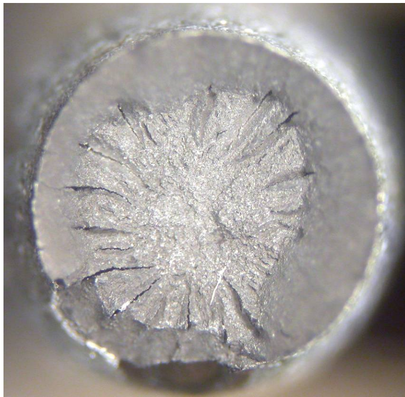
Fig.16 Wire 1-4 surface (top) and fracture surface after tensile testing (bottom).
