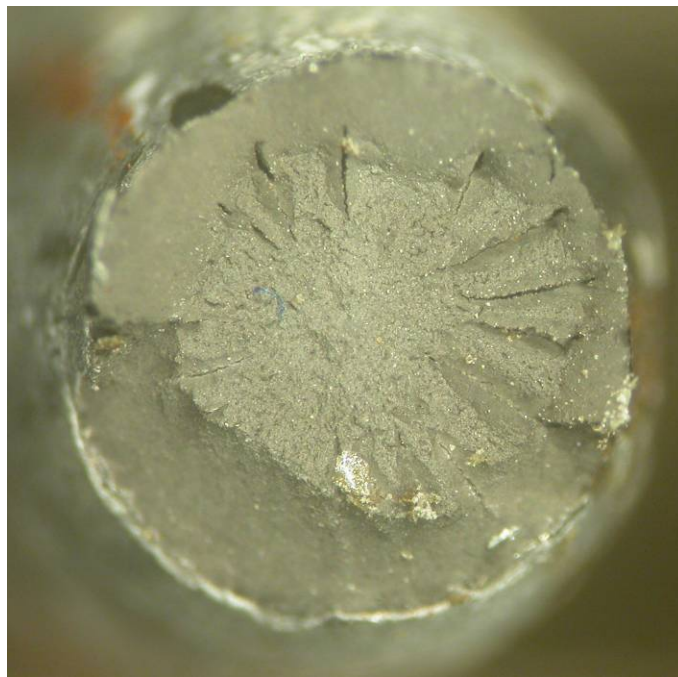
Fig. 63 Wire 9-3 surface (top) and fracture surface after tensile testing (bottom).
