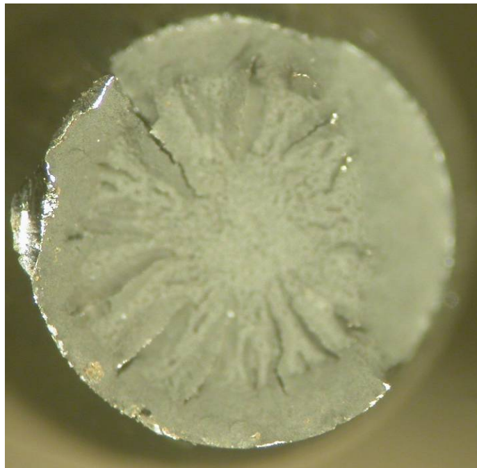
Fig. 87 Wire 12-4 surface (top) and fracture surface after tensile testing (bottom).
