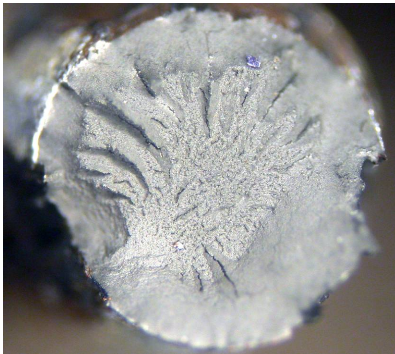
Fig. 42 Wire 5-7 surface (top) and fracture surface after tensile testing (bottom).
