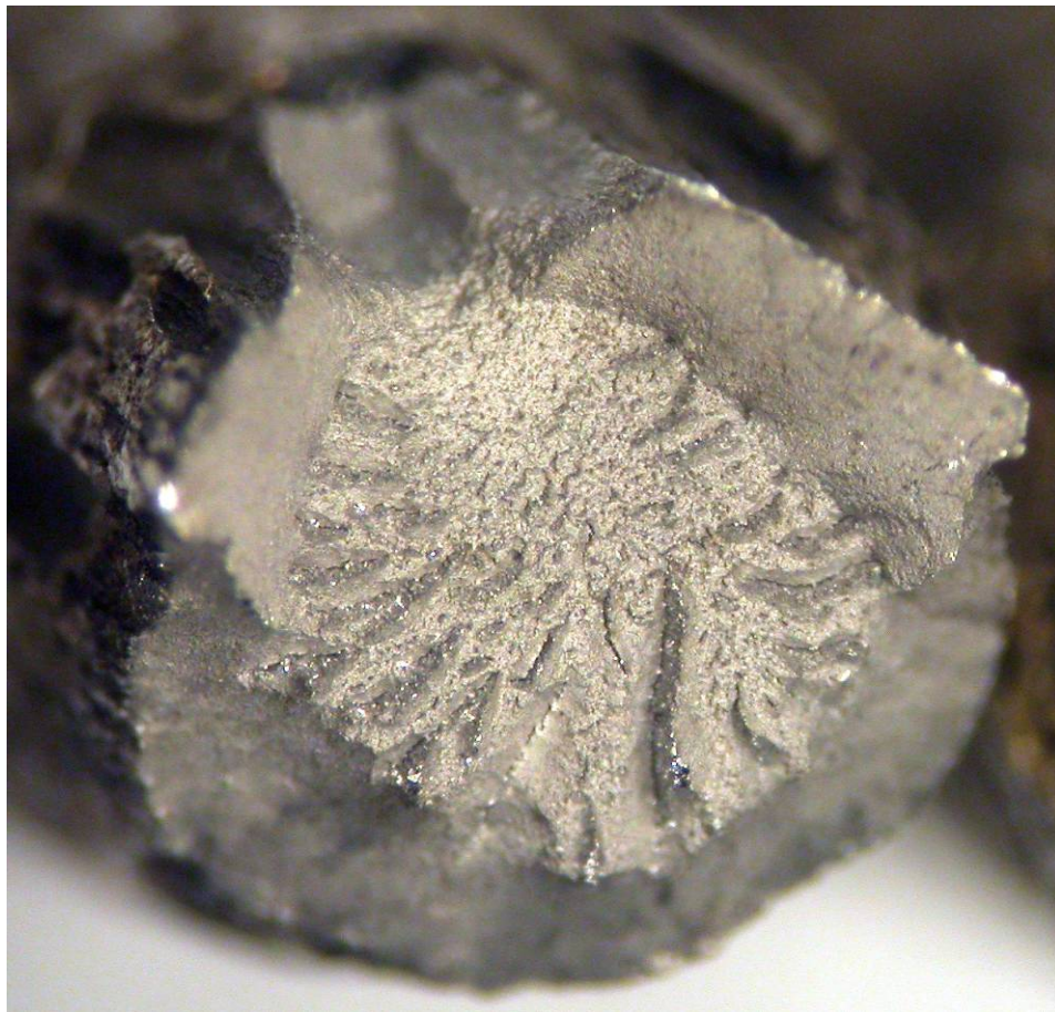
Fig. 52 Wire 7-4 surface (top) and fracture surface after tensile testing (bottom).
