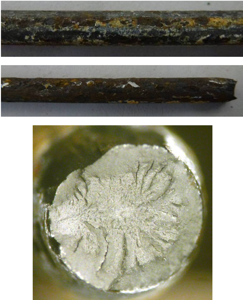
Fig. 49 Wire 7-1 surface (top) and fracture surface after tensile testing (bottom).
