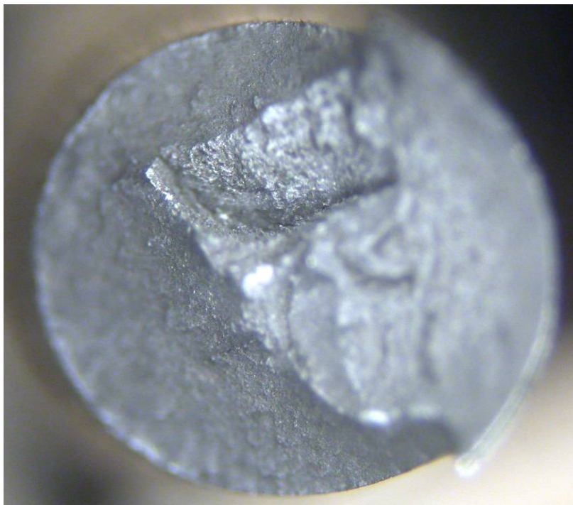
Fig. 19 Wire 2-1 surface (top) and fracture surface after tensile testing (bottom).
