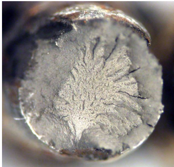
Fig. 102 Wire 5-7 fracture profile (top) and fracture surfaces (bottom).
