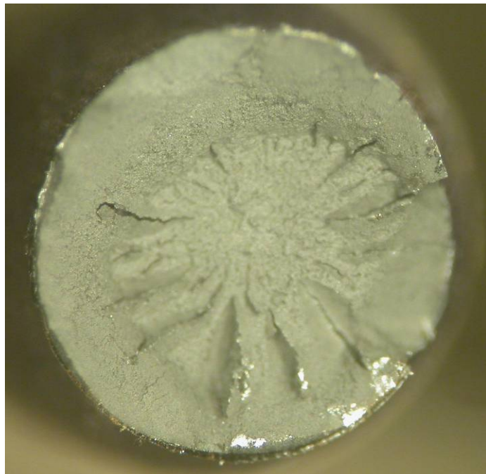
Fig. 83 Wire 11-6 surface (top) and fracture surface after tensile testing (bottom).
