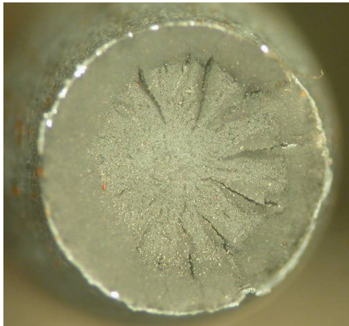
Fig. 70 Wire 10-4 surface (top) and fracture surface after tensile testing (bottom).
