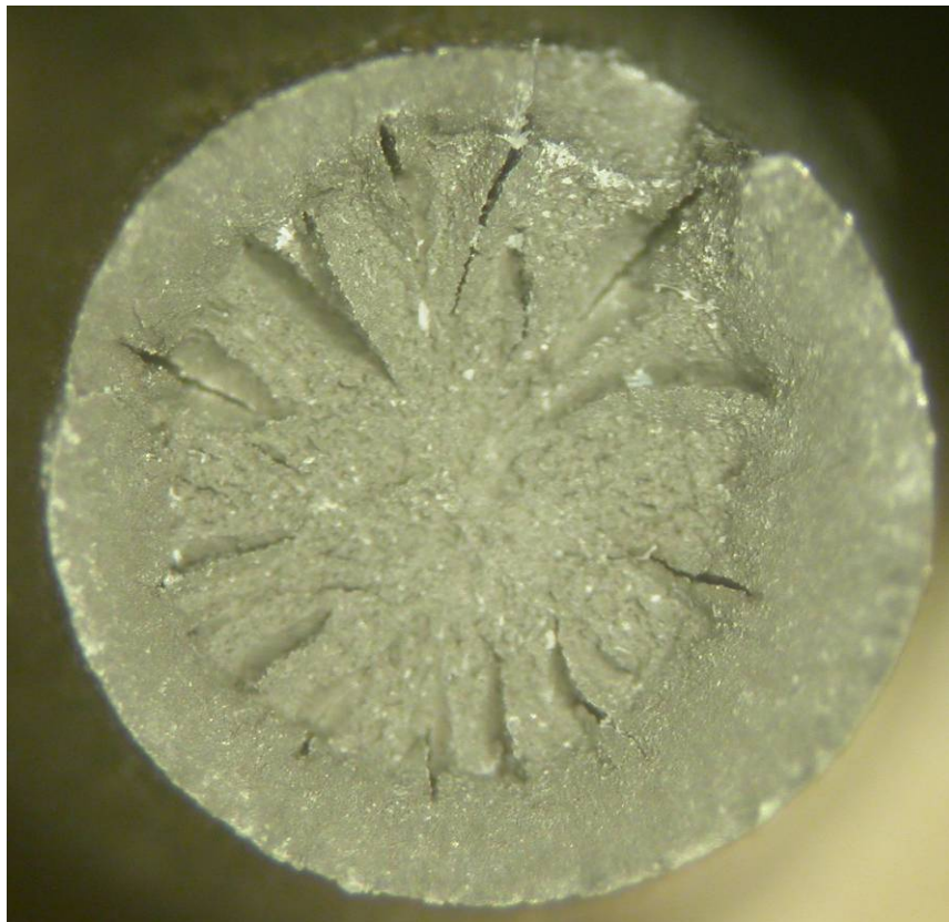
Fig. 67 Wire 10-1 surface (top) and fracture surface after tensile testing (bottom).
