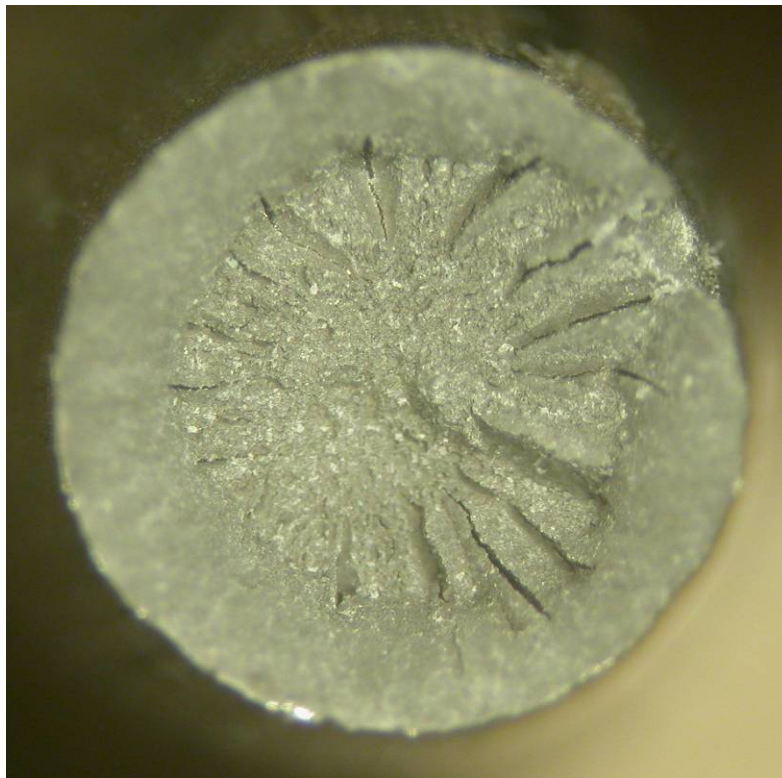
Fig. 65 Wire 9-5 surface (top) and fracture surface after tensile testing (bottom).
