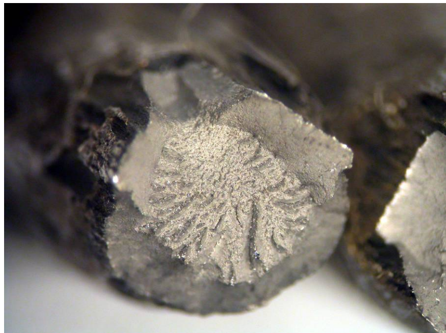
Fig. 104 Wire 7-4 fracture profile (top) and fracture surfaces (bottom).
