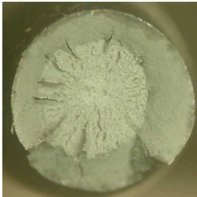
Fig. 77 Wire 10-11 surface (top) and fracture surface after tensile testing (bottom).
