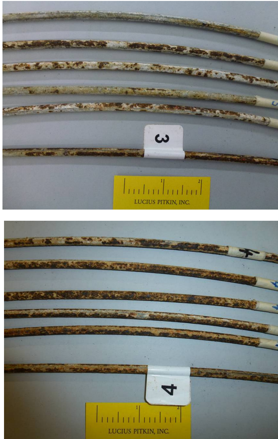
Fig. 5 Views of wire 3 and 4 surfaces (see Table 2).
