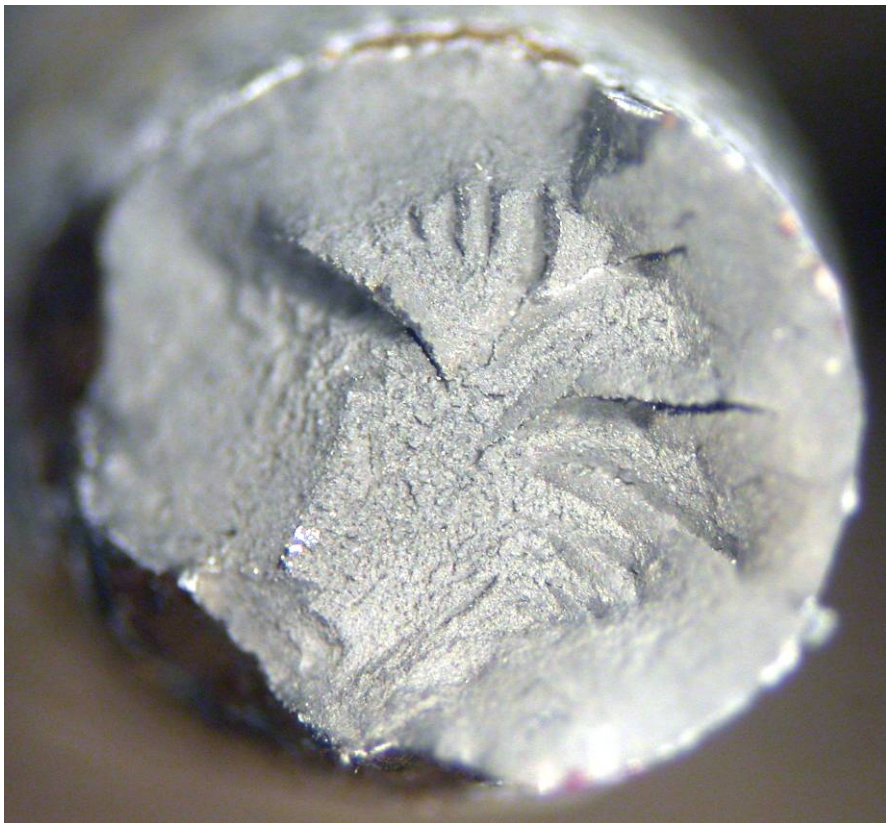
Fig. 29 Wire 3-6 surface (top) and fracture surface after tensile testing (bottom).
