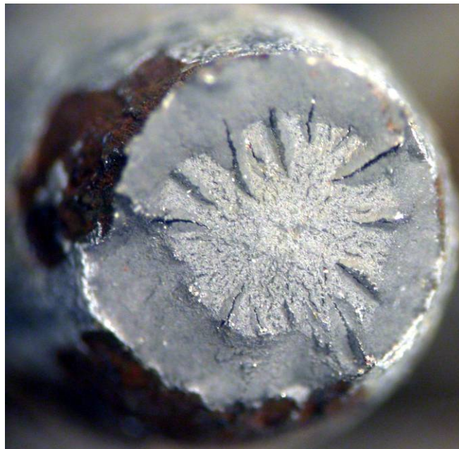
Fig. 108 Wire 6-4 fracture profile (top) and fracture surfaces (bottom).
