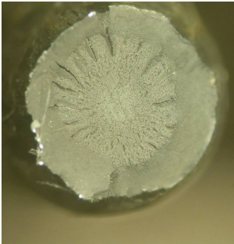
Fig. 60 Wire 8-6 surface (top) and fracture surface after tensile testing (bottom).
