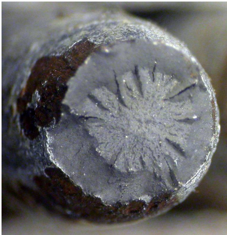
Fig. 47 Wire 6-4 surface (top) and fracture surface after tensile testing (bottom).
