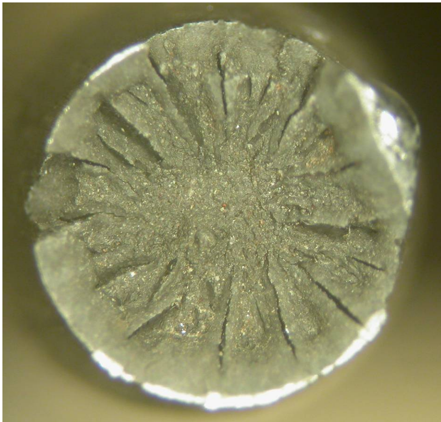
Fig.15 Wire 1-3 surface (top) and fracture surface after tensile testing (bottom).
