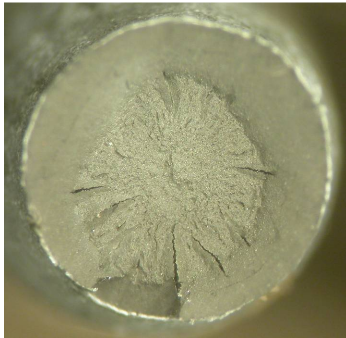
Fig. 94 Wire 13-4 surface (top) and fracture surface after tensile testing (bottom).
