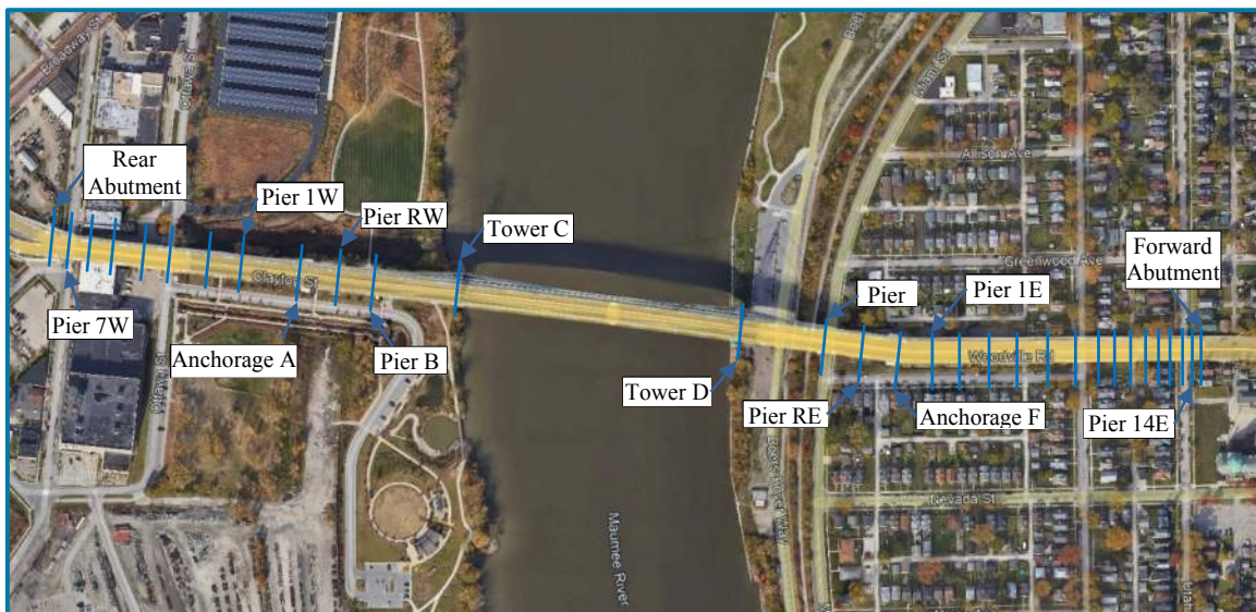
Figure 2 – Plan View and Bridge Nomenclature
