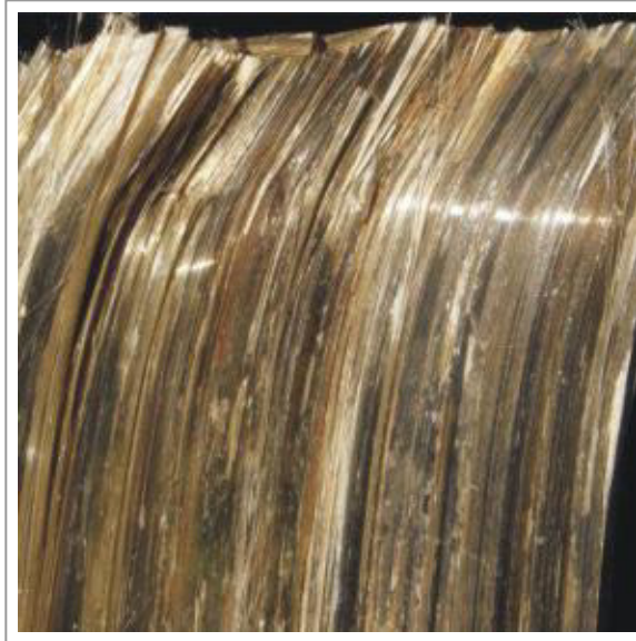
Amosite – Brown asbestos
