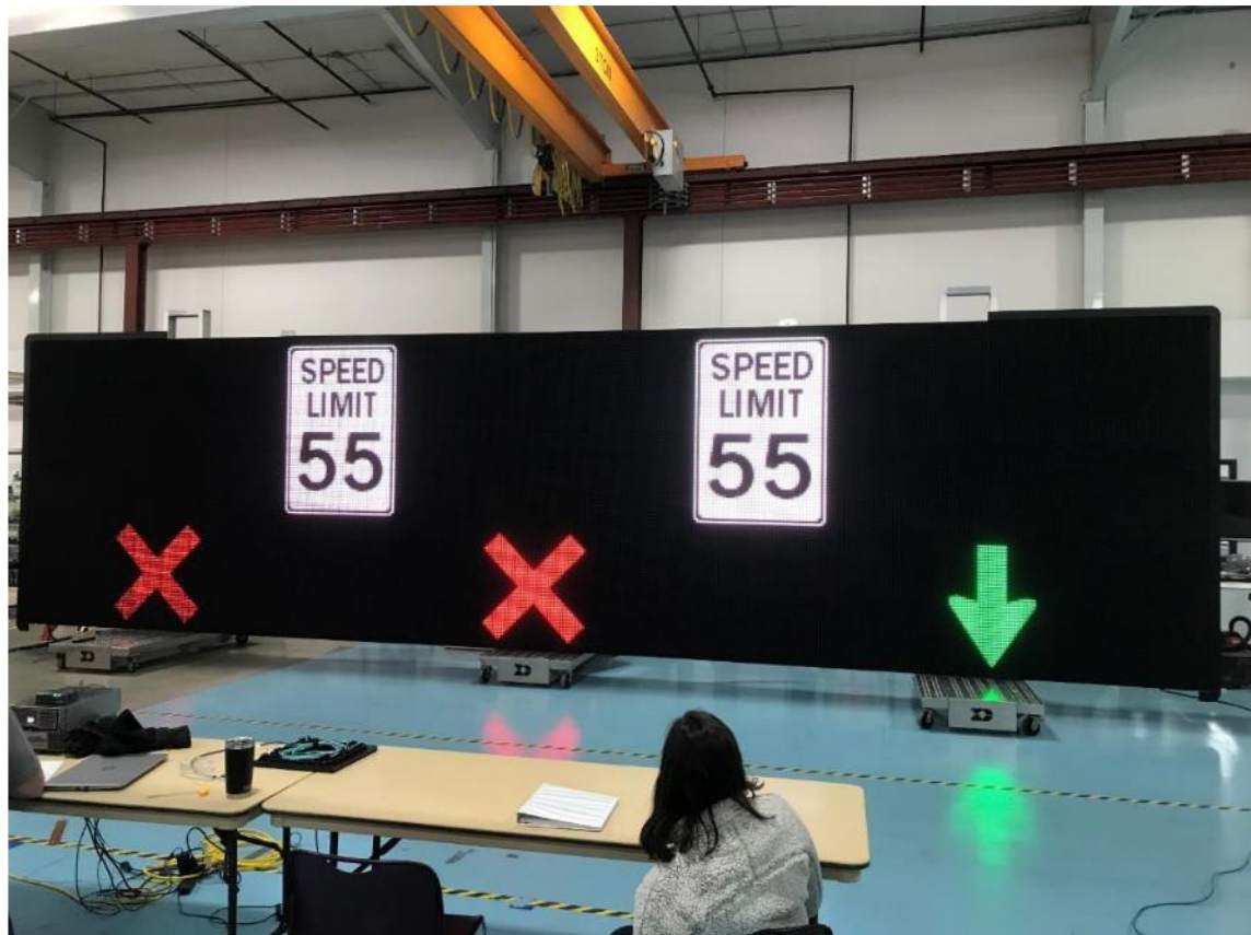
Figure 1-8. DMS Factory Acceptance Testing for Part-Time Shoulder Use + Lane Control + Variable Speed Limits
