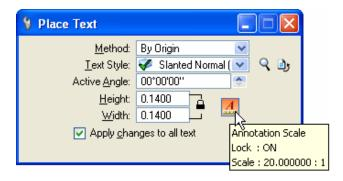
In the example above, the ODOT, standard text style **Slanted-Normal LS=0.50** has been selected with the Model annotation scale set to **Engr 1:20**. The text size and line spacing will be set as follows:
