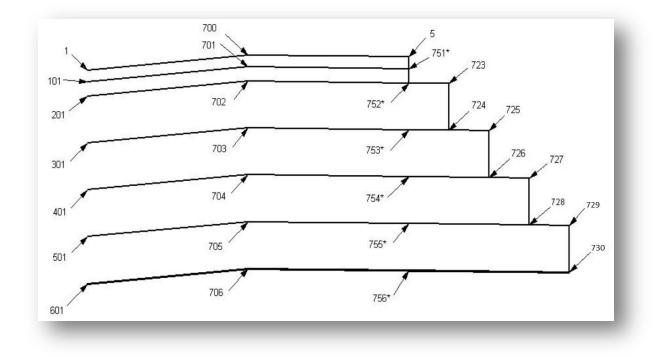
After processing the shoulder, marked points 101, 201, 301, 401, 501, and 601 are relocated at the edge of the shoulder corresponding with points 751, 752, 753, 754, 755, and 756.
