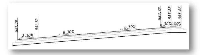
On the high side of superelevation, the criteria will break the shoulder slope as shown above.
