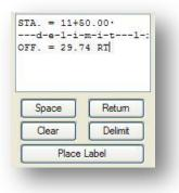
The **Label Edit Field**, located in the upper right portion of the dialog, reflects the text in the current label. Labels can be constructed by any combination of **Computed Text**, **Inserts**, **User Inserts**, or manually typed text strings.
