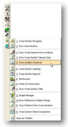
The application can also be accessed by selecting **Applications > Road > Cross Sections > Draw Ancillary Features** from the MicroStation pull-down menu.
