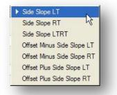
The **Side Slope LT** and **Side Slope RT** conditions are used to define the criteria files for the Left and Right sides of the pavement slopes separately. If the same list of criteria files is to be processed on both the Left and Right side of the roadway, the **Side Slope LTRT** condition may be used.
