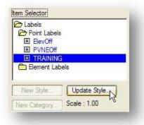
After modifying a style, the user may want to save the current modifications. Simply press the **Update Style** button to invoke the dialog depicted below. Both **Before** and **After** labels are shown, so the user can easily discern the changes.
