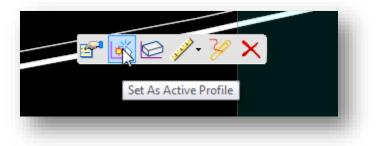
When the command is selected, the cable barrier is automatically adjusted to use the new profile.
