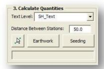
This option is used to add end area, or end width, quantities together to generate the earthwork and seeding quantities.
