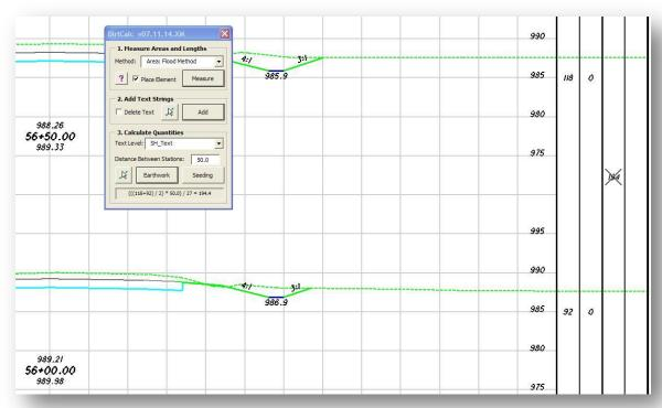
The quantity calculation is shown at the bottom of the dialog box.
