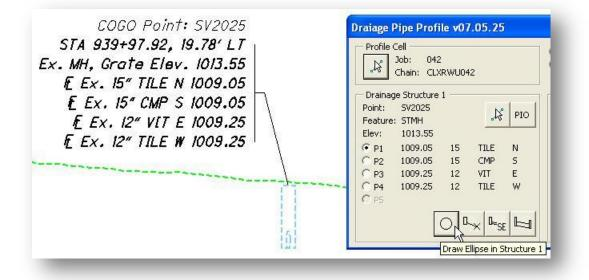
The **Draw Ellipse** button is used to draw an ellipse, representing the selected pipe, in the profile. In the example above, the 15" Tile pipe is drawn in the profile when the **Draw Ellipse** button is selected.
