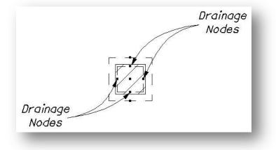
When the pipes are drawn using the ODOT VBA application **ODOT\_DrainagePlan2.mvba**, the pipes are connected from node to node as shown in the example below.
