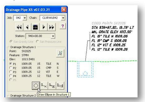
The **Draw Ellipse** button is used to draw an ellipse, representing the selected pipe, in the cross section. In the example above, the 15" TILE pipe was is selected and was drawn in the cross section when the **Draw Ellipse** button was selected.
