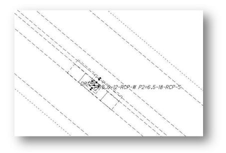
Example 4: Rotating cells relative to a GEOPAK Chain
