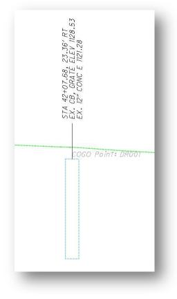
The **Move Label** option is used to move previous placed labels. The label and the leader lines are manipulated as one group using this command.
