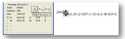
The elevation for each pipe is calculated by subtracting the *dip* value from the point elevation. For example, point DR002 was stored with an elevation of 1030.25 in the example above. The parameters for pipe P1 were defined are as follows:
