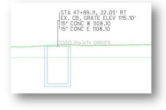
The drainage structure outline is tagged with a GEOPAK Adhoc attribute that is used by the **ODOT\_DrainageXS2.mvba** application to draw the pipes between the structures on the cross section. Select the *GEOPAK Application Attribute Viewer* to view the Adhoc attribute information.
