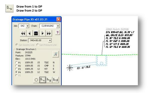
The **Draw to DP** buttons are used to draw the selected pipe to a data point location as shown in the example above.
