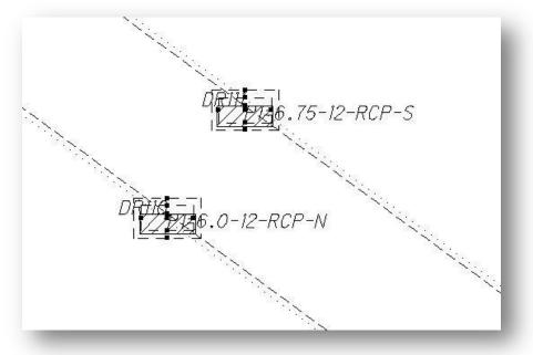
Rotating curb inlets is a little different than rotating catch basins. The grate of the cell should be inside the pavement. Rotating both cells in the example above relative to the edge of pavement will result in the grate for the cells on one side of the pavement falling on the wrong side of the curb. For this reason, it is necessary to rotate the inlet cells on each side of the roadway separately. The following steps are used to rotate the cells for the median inlets.
