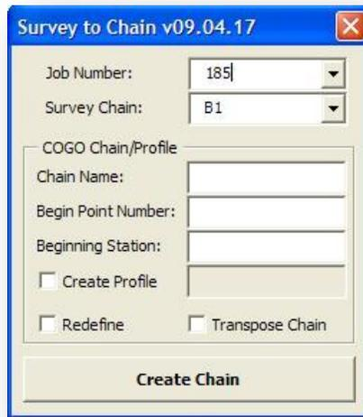
The application searches the current GEOPAK Working Directory for GPK files. If a GPK file is found, it is listed in the **Job Number** drop down list and the list of **Survey Chains** is populated. The application automatically adjusts the MicroStation view window to display the first survey chain in the selected GPK file.
