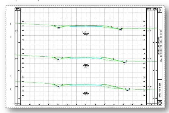
Notice that the existing ground line extends through the quantity columns on the completed sheets. Users may wish to partial delete the ground line in the original cross section cell file so that it falls within the limits of the boarder element as shown in the example below.
