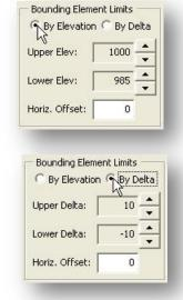
When **By Elevation** is selected, the **Upper Elev** and **Lower Elev** values are used to set the upper and lower elevation limits of the boundary element. Selecting the up and down arrows to the right of each field will increase or decrease by the **XS Scale** value.
