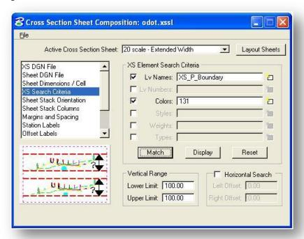
When clipping cross section sheets with GEOPAK, the **XS Search Criteria** item is used to select the level symbology for the MicroStation graphics that will be used to define the vertical limits of each cross section. There are several advantages to using a bounding element to define the **XS Search Criteria**:
