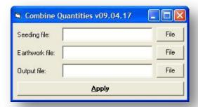
Select the GEOPAK **Seeding File** and the **Earthwork File** to combine. Key-in the name of the **Output file** to be created by the application. Select **Apply** to append the seeding quantities to the earthwork quantities and generate the new output file. An example of the combined quantities is shown below:
