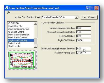
The **Left Clip X Offset** and **Right Clip X Offset** values have been adjusted in ODOT.xssl to include the width of the quantity columns.
