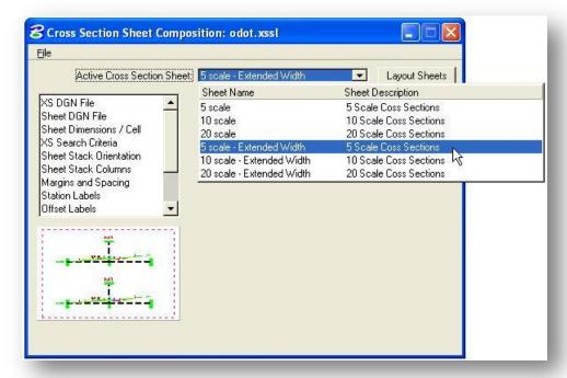
For each of these three options, the width of the clipping area has been extended to include the seeding and earthworks quantity columns within the reference boundaries for each cross section.
