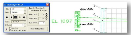
The **Horiz. Offset** key-in field is used to enter an offset value to shift the XS Boundary to the left or right as shown in the example below. Use this option to align the boundary with the cross section sheet layout when the completed cross sections will be shifted off center on the completed sheets. The value of the **Horiz. Offset** is multiplied by the **XS Scale** to determine the offset in the design file.
