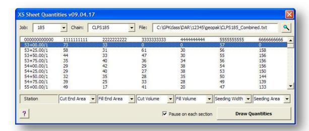
The quantity values contained in columns 1, 2, 3, and 4 are user definable when the original earthworks quantity file is generated with GEOPAK. The <u>ODOT GEOPAK Road 2</u> training guide recommends defining the columns in the following order:
