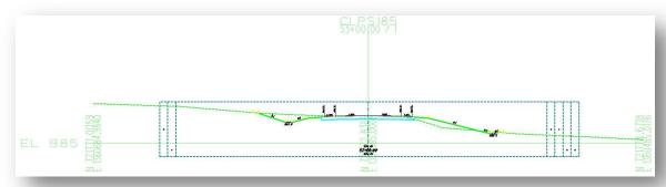
The boundary element is drawn at the width of a standard ODOT Cross section sheet cell and includes columns for the cross section quantities. The bounding element is intended to be used when clipping cross section sheets to set the **XS Search Criteria** as shown in the example below.
