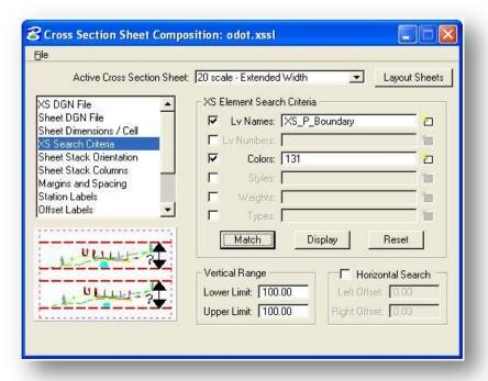
Note that the **XS Search Criteria** is only used to set the vertical extents of each cross section on the completed sheets. The horizontal limits are set in the **Margins and Spacing** item shown below.
