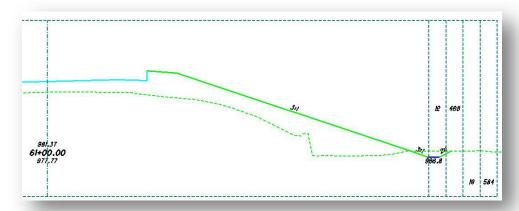
Use the boundary element with a grid to facilitate breaking up the cross section into a match line segment as shown in the example below.
