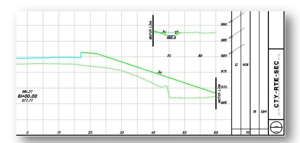
**Note:** The elevations on the side of the cross section sheet are placed by GEOPAK for the vertical extent of the boundary element. In the case where match lines are included within the clipping limits of these elevations must be manually edited to reflect the correct elevation values of the match line segment.
