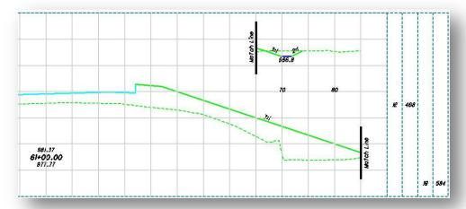
The boundary element is used to define the vertical extents of the cross section on the completed sheet. The example on the following page shows the cross section on the completed sheet.
