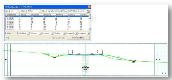
If a set of quantities has been previously placed for the cross section(s) using this application, the previously placed quantities will be automatically deleted from the cross section(s).
