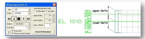
If the reference elevation is not evenly divisible by the **XS Scale**, a horizontal grid line is inserted about the reference elevation and the **Upper Delta** and **Lower Delta** values are measured from the extra grid line as shown in the example below. This is necessary to ensure that the grid interval matches the **XS Scale** value.
