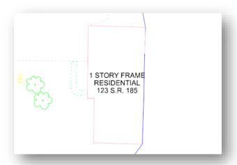
Annotations can be removed by manually deleting the text, or by use of the **Remove Element Annotation** or the **Remove Model Annotations** command.
