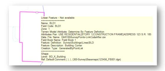
The **Feature Definition** assigned to the element controls how each Survey item is annotated. The annotation is also depended on whether the surveyor entered any attribute data in the field as the survey data is collected.
