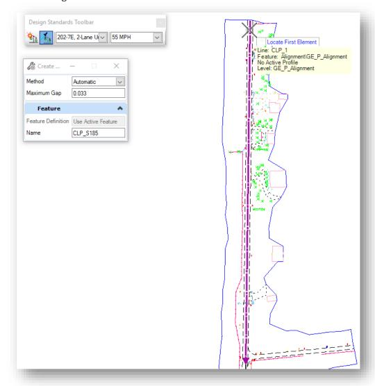
The chain is stored with a default beginning station value of 0+00. Use the **Start Station** tool to define the beginning station for the newly created alignment as detailed below.
