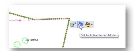
✓ From the **Geometry** tab, choose **Standards** > **Features Definition Toolbar**. Set the active feature to **Alignments** > **GE\_P\_Alignment**. Toggle on the **Use Active Feature Definition** icon.
