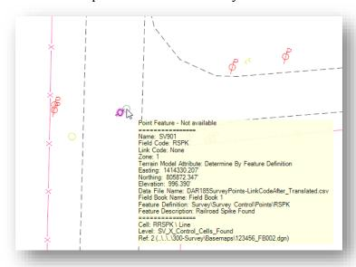
Use the MicroStation **Origin Snap** to ensure you are starting the first point of the line by snapping to the origin of the RRSKP cell.
