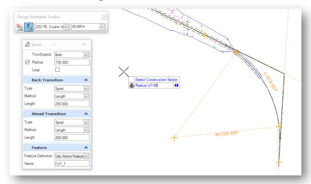
**Tip:** The degree of curve can be set by keying in the degree value in the **Radius** field prefixed with a lower case "d". Degrees, minutes, and seconds are separated by the colon character.
