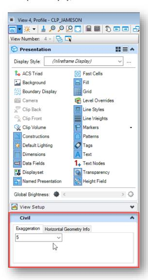
To change the profile display exaggeration factor, select the desired exaggeration factor from the drop-down list.
