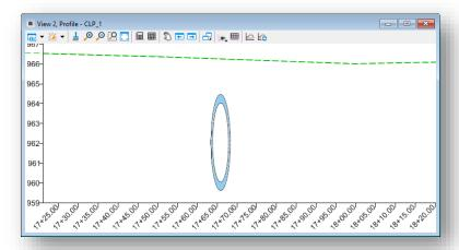
The 3d Cut graphics are a static representation of the elements in the 3d model at the time the 3d cut graphics were generated. To update the 3d cut graphics, the following commands are available in the Profile View window.
