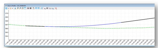
There are cases where the user may need to display the profile information using different symbology other than the parameters defined with the horizontal geometry feature definition. The OHDOT WorkSpace includes additional features for profiles in the **Linear > Profiles** category as shown below.
