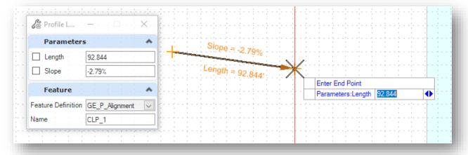
The feature definition is defined to differentiate between the tangent lines and vertical curves. Proposed profiles are defined to display the vertical curves with color 58, and tangent lines with color 0, as shown below.
