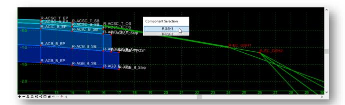
✓ Delete the 4:1 fill slope component on each side of the template. The completed template should appear as shown below.
