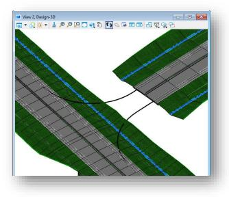
The profile for each radius return can be reviewed and edited by selecting one of the radius returns and selecting the **Open Profile Model** command. The profile for **R-Radius St Peter Road** is shown below.
