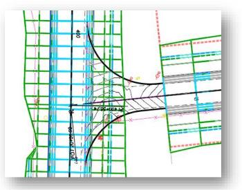
The process to define the pavement buildup, add the shoulder and side slopes, and trim the S.R. 185 corridor model through the limits of the intersection are detailed in Parts 2, 3, & 4 of Exercise 2.
