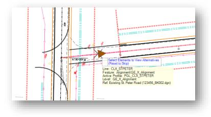
The edge of pavement element can also be reversed by left-clicking the edge of pavement line.
