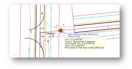
Left-clicking on the center line of St. Peter Road will reverse the direction of the element for the civil cell placement as shown below.
