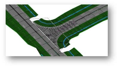
Depending on the template drop interval and the location of the radius returns, there may be a gap in the model as shown above. This can be remedied by inserting a key station on the S.R. 185 corridor to ensure that the model is processed up to the station where the radius return starts.
