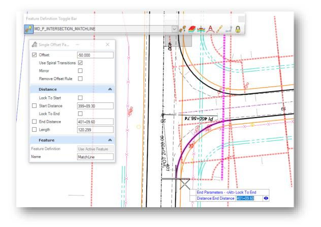
The match line element must be added as a corridor reference to the S.R. 185 corridor for the template to find the graphic. Take the following steps to add the match line element as a corridor reference:
