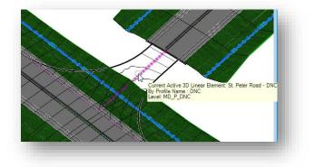
Add this new partial offset line to the surface terrain model as a break line.
