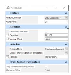
• Next if a reference element as selected you can enter a vertical offset from that reference element. If a reference element was not selected, you can enter the desired elevation.
