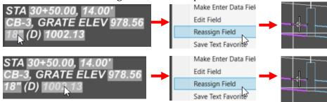
• The (D) standards for direction and has to be manually typed in. This is the direction the pipe is going away from the node.
