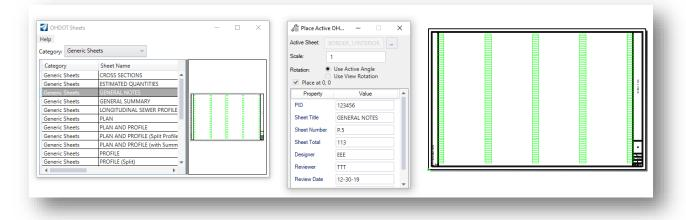
The OHDOT sheet seeds files, which are used as the seed file when the sheet design file is created, are configured with the **Show Sheet Boundary** parameter set to a value of **True**. The boundary can be used for the sheet border placement by snapping to the lower left corner of the boundary. In the example above, the sheet is placed at the (0,0) coordinate location using the **Place at 0,0** option.
