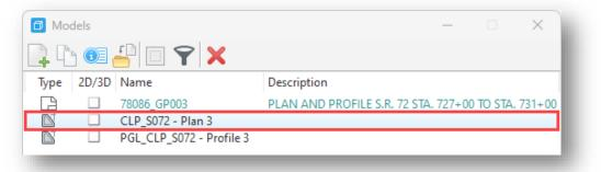
• Activate the plan view drawing model by double-clicking the model's name (CLP\_S072 – Plan 3) in the **Models** dialog.
