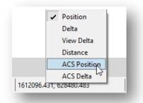
As the cursor is moved in the view window, the ACS coordinates are displayed in Longitude (Easting), Latitude (Northing) format as shown below.
