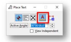
With the **Annotation Scale** parameter toggled on, text is placed in the file using the current annotation scale value as a multiplier.
