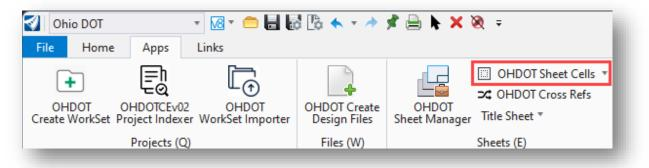
Cells that have interior components, such as the title sheet, are split into two separate cells: one for the border and one for the interior. Placement of the sheet cell border and interior is facilitated by use of the **OHDOT Sheet Cells** application.
