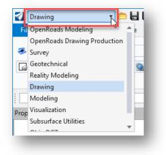
The **WorkFlows** present the various ORD commands logically organized according to a task. For example, the **Drawing** workflow contains commands that are used for typical MicroStation drawing tasks.
