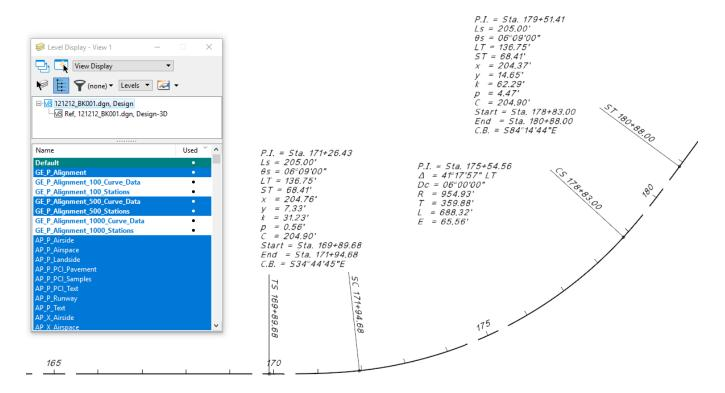
**Note:** The levels are named according to the station label intervals (100', 500', and 1000'), not the annotation scale value. For example, the **GE\_P\_100\_Stations** and **GE\_P\_100\_Curve\_Data** levels are appropriate for multiple annotation scale values (1:10, 1:20, 1:50).
