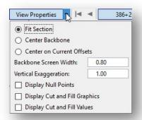
The **View Properties** contains parameters for adjusting the cross-section display, as shown at left.
