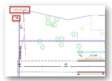
The template range can be edited by selecting the station and editing the value of by selecting the arrow icon to dynamically mode the start (or end) of the template range.
