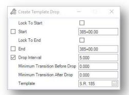
The parameters can be defined in the *Crete Template Drop* window, as shown at left, or by dialogs floating on the cursor that will step you through the parameters.
