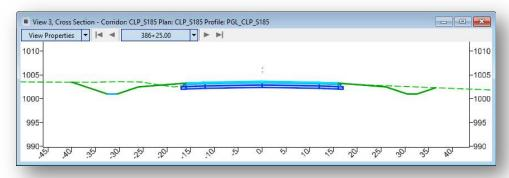
This dynamic view is a temporary display of the cross sections. The sections are not written to the design file using this command.
