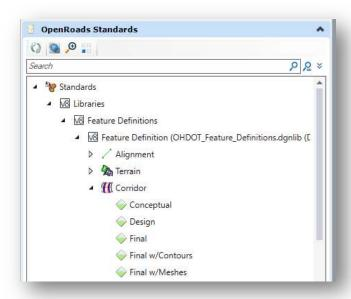
The feature definition assigned to a corridor can be changed at any time throughout the corridor modeling process.
