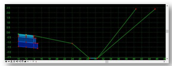
The shoulder components are currently located 10' right of the origin. The next step is to move the shoulder to the 0.0 origin in the template dialog.
