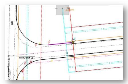
✓ To adjust the civil cell, select the civil cell element that overlays the St. Peter Road alignment. The length of the civil cell is a rule that can be edited (the value is 100.000' in the example below), or the length can be dynamically modified by choosing the left arrow at the end of the civil cell and dragging the length to the desired location.
