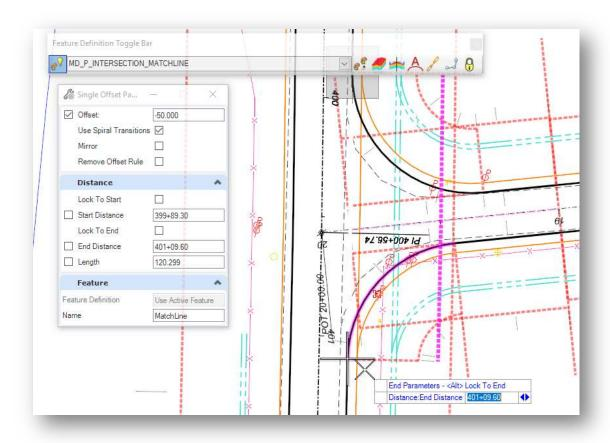
The match line element must be added as a corridor reference to the S.R. 185 corridor for the template to find the graphic. Take the following steps to add the match line element as a corridor reference:
