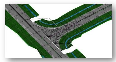
Depending on the template drop interval and the location of the radius returns, there may be a gap in the model as shown above. This can be remedied by inserting a key station on the S.R. 185 corridor to ensure that the model is processed up to the station where the radius return starts.
