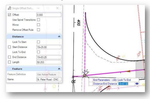
After placing the line, assign a profile to the line using the **Profile By Slope From Element** command.
