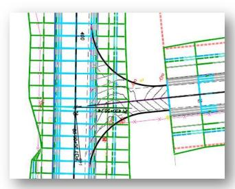
The process to define the pavement buildup, add the shoulder and side slopes, and trim the S.R. 185 corridor model through the limits of the intersection are detailed in Parts 2, 3, & 4 of Exercise 2.
