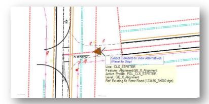
Left-clicking on the center line of St. Peter Road will reverse the direction of the element for the civil cell placement as shown below.
