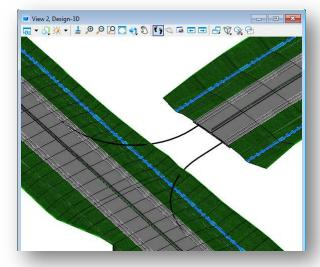
The profile for each radius return can be reviewed and edited by selecting one of the radii returns and selecting the **Open Profile Model** command. The profile for **R-Radius St Peter Road** is shown below.
