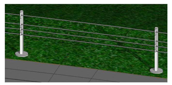
In the example above, the cable barrier was placed at an offset of 1.0' from the edge of shoulder.
