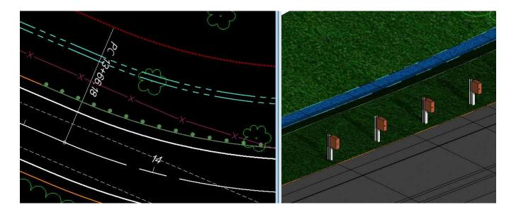
The rail is placed using the **Model Detailing > Apply Linear Template** command to assign the template to the guardrail run in the 2D view.
