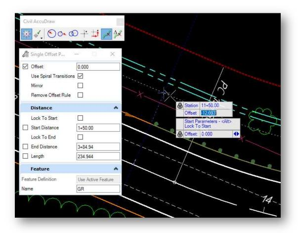
Since the edge of shoulder element does not have stationing assigned, the centerline will be used as the reference element to define the station value. **Civil AccuDraw** is used to facilitate this task.
