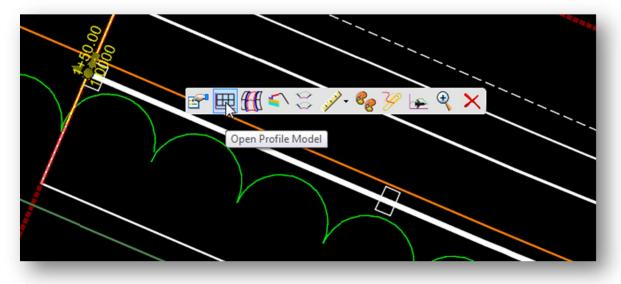
• When prompted, open a new view window, and issue a data point in the view to display the profiles for the cable barrier element. An example is shown below.
