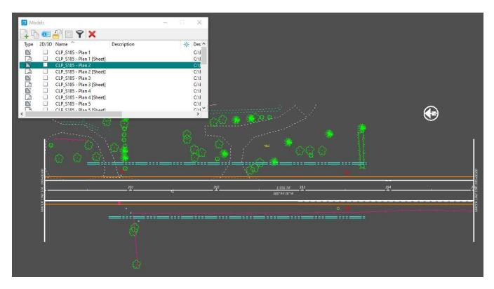
The drawing models are referenced to a sheet model with a sheet border to assemble the completed sheets for plotting and PDF generation as shown in the example below.
