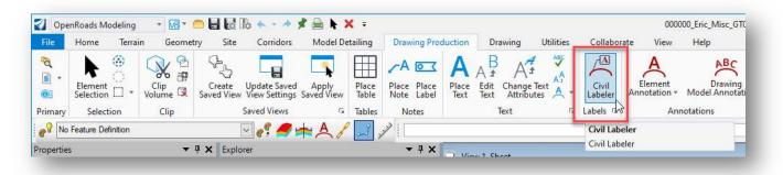
When the command is selected, the *Civil Labeler Tool* dialog is opened with the **OHDOT\_Civil\_Labeler.xml** file loaded as shown below.
