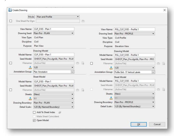
✓ Toggle on the **One Sheet Per Dgn** option if you desire to create a new design file for each sheet. When this option is toggled on, the name entered for the plan view **Sheet Model > Model Name** parameter is used to create each sheet design file.
