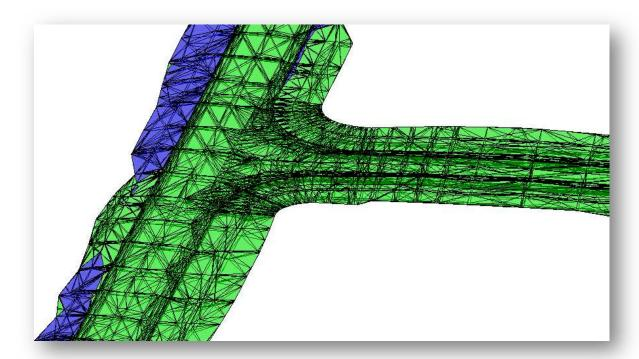
The 3D mesh elements are generated in the **Roadway Digital Terrain Model** file type.
