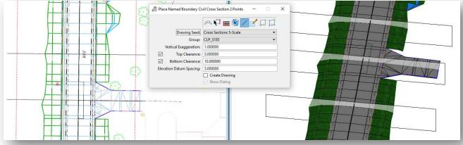
**Tip:** For best results, create any additional named boundaries using Civil AccuDraw to define the station and offset values for the boundary. Use the same offset values as the primary cross-sections.
