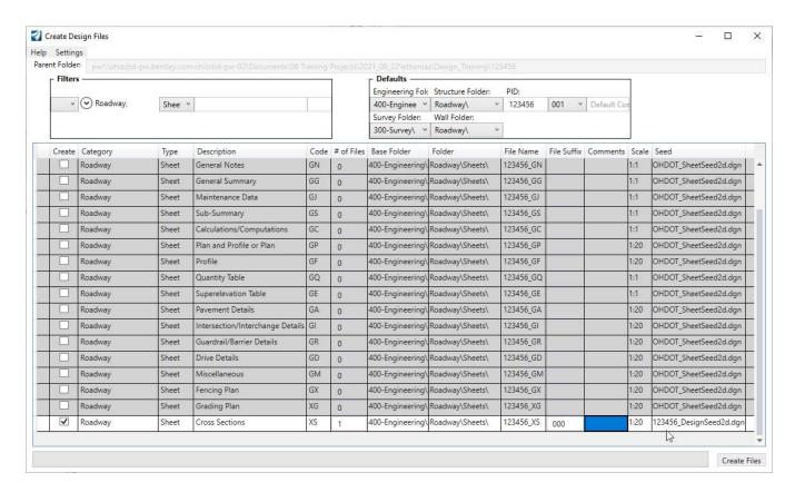
In the example above, the file suffix of **000** has been entered for the **Cross Sections** sheet type. The application recognizes the 000, 100, 200, etc. series as container files and has automatically switched the **Seed** file to the appropriate design seed for the WorkSet.
