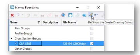
3. Choose the **Create Cross Section Drawing** command. The *Create Drawing* dialog, previously described, is opened. Complete the *Create Drawing* dialog to generate the cross-section sheets.
