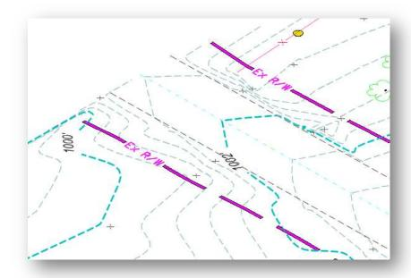
When cross sections are generated, if the cross section intersects a 3D Right-of-Way line in the 3D model, a cell is placed in the cross section at the right-of-way line offset and elevation.
