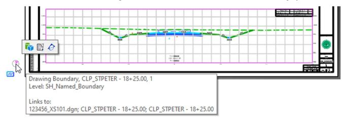
Saved Views quick access dialog icons. This can be used to navigate between the cross sections from the sheet models.
