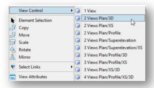
The graphics that will be displayed on the clipped cross sections are controlled by what is displayed in the 3D view. Toggle on/off the desired levels in the 3D view before proceeding.
