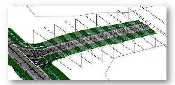
Before generating the named boundaries, a design file is created as a "container file" to attach references and place the named boundaries for the cross-section locations. The 3D model must be displayed in order to place the named boundaries. The cross section are cut from the 3D model. In the example above, the geometry, survey, and corridor model basemaps are attached to the plan view with the 3D model displayed. The named boundaries are placed in the 3D model relative to a selected alignment.
