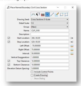
The boundaries are drawn for the cross sections and the *Placed Named Boundary* dialog is closed.
