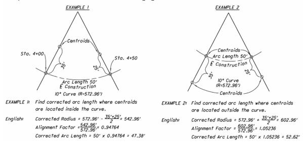
The diagram of the example showing the method of correction should be shown on the General Note Sheet. The corrected arc lengths should be shown in the earthwork tabulations on the cross-section sheets.
