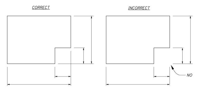
Extension lines should not be shortened. Also, a dimension line should never coincide with or form a continuation of any line of the drawing. If possible, dimensions should always be placed off the object.
