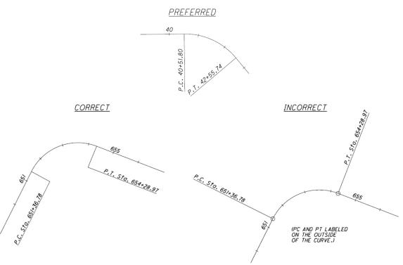
When space prohibits or when an alignment has a large number of horizontal curves, label each curve and tabulate the curve data. If it is necessary to tabulate curve data for a few curves along an alignment, then all curves should be tabulated to provide consistency.
