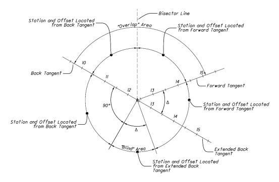
In addition to the "overlap" area, there is a "blind" area in which a station and offset cannot be measured from either the back or forward tangent. Stations and offsets in the "blind" area should be measured off an extended back tangent as shown in the figure.
