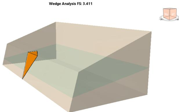
Figure 8: Critical wedge within described geometry
