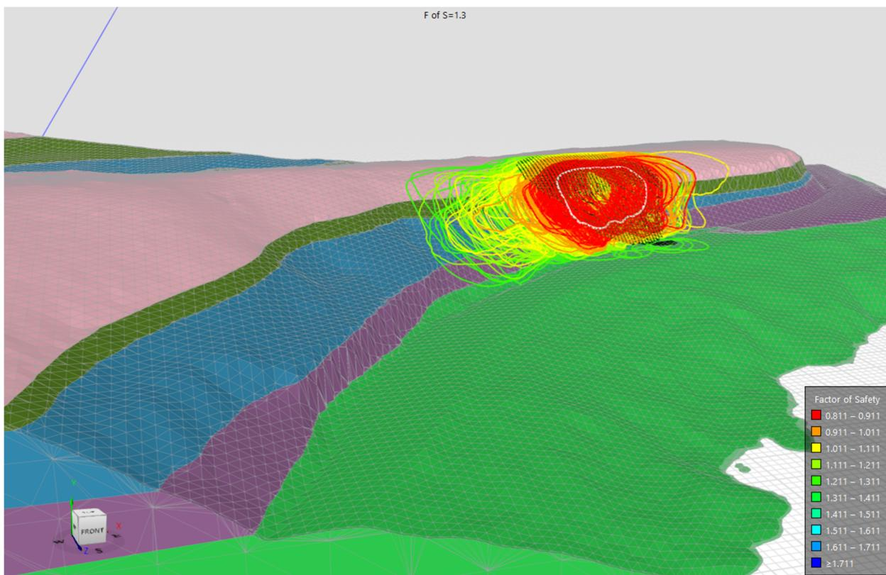
Figure 10: View of failure circles along SR 13, looking West
