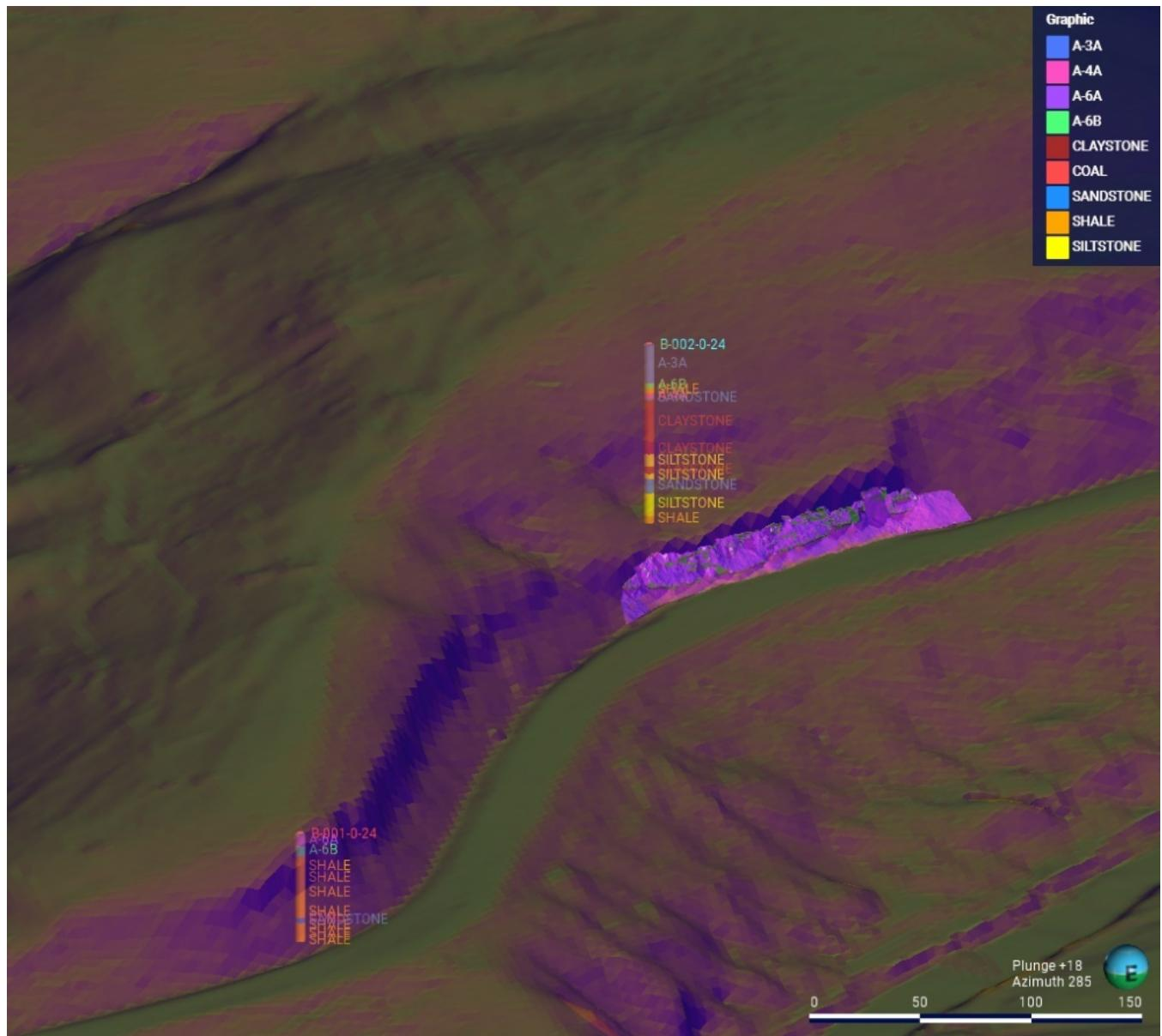
**Figure 4: View of as-drilled boring locations on 3D topography**
