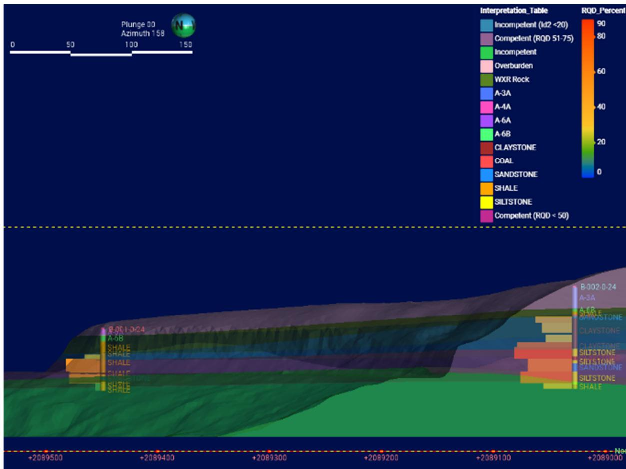
Figure 6: Cross sectional view of geologic model adjacent to B-002-0-24 with Strata and RQD plotted downhole
