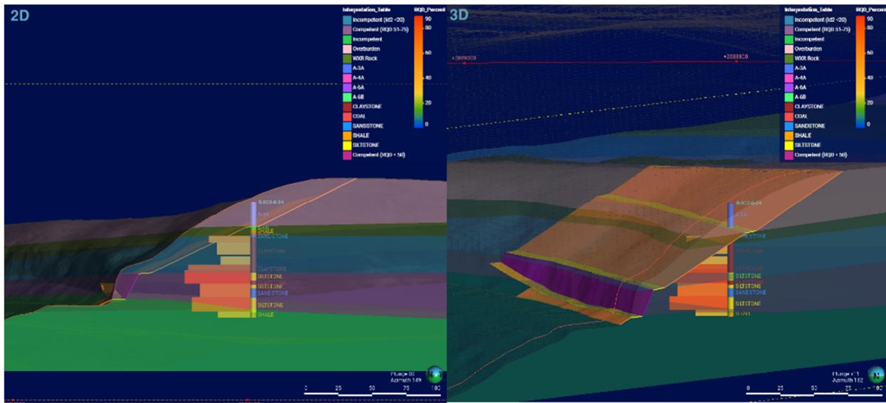
Figure 12: 2D and 3D view of geologic model at critical section with proposed geometry
