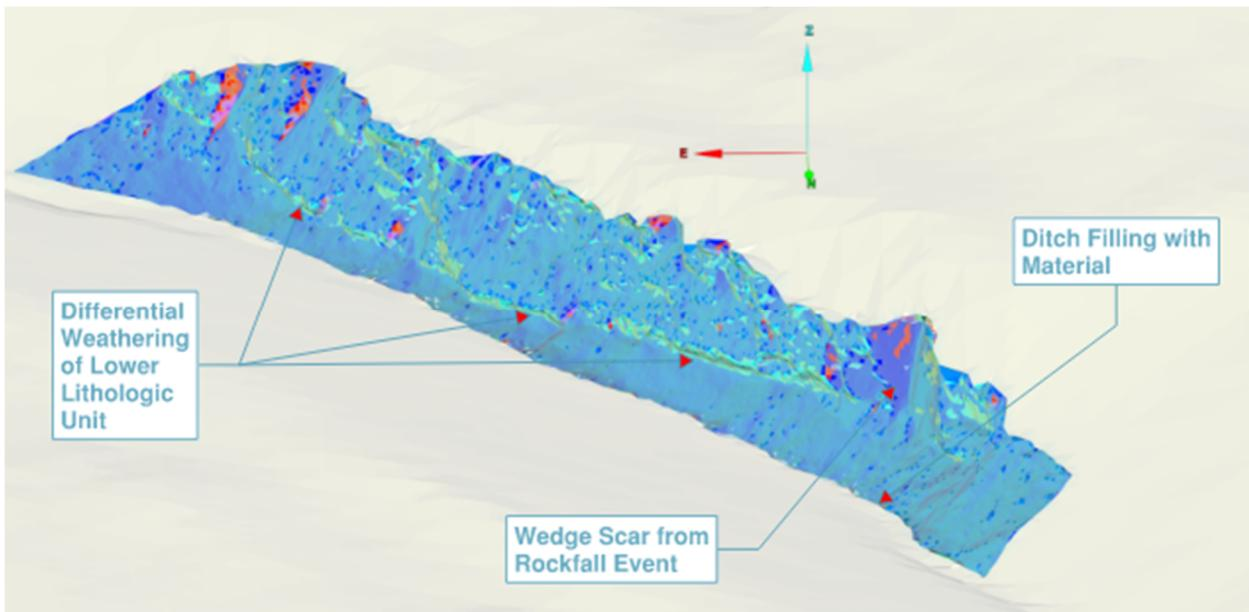
Figure 2: Annotated view of detailed rock slope LiDAR
