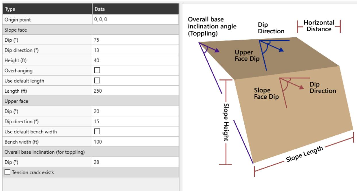
Figure 7: Critical block section geometry
