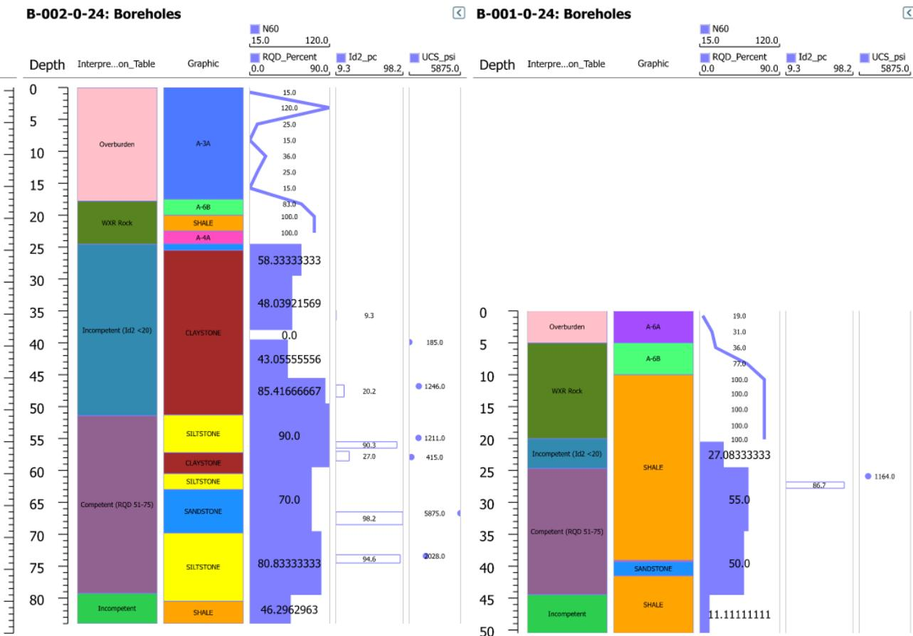
**Figure 5: Interpreted profile showing interpreted rock slope design units alongside strata, N60, RQD, SDI and UCS values**
