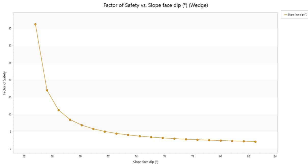
Figure 9: Sensitivity analysis of slope face dip against Factor of Safety
